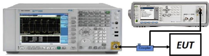
Figure 7-4. Test Instrument & Measurement Setup
