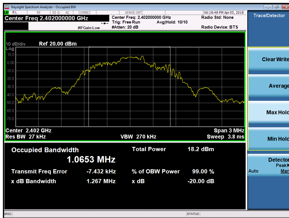
Plot 7-1. 20dB Bandwidth Plot (Bluetooth, 1Mbps – Ch. 0)
