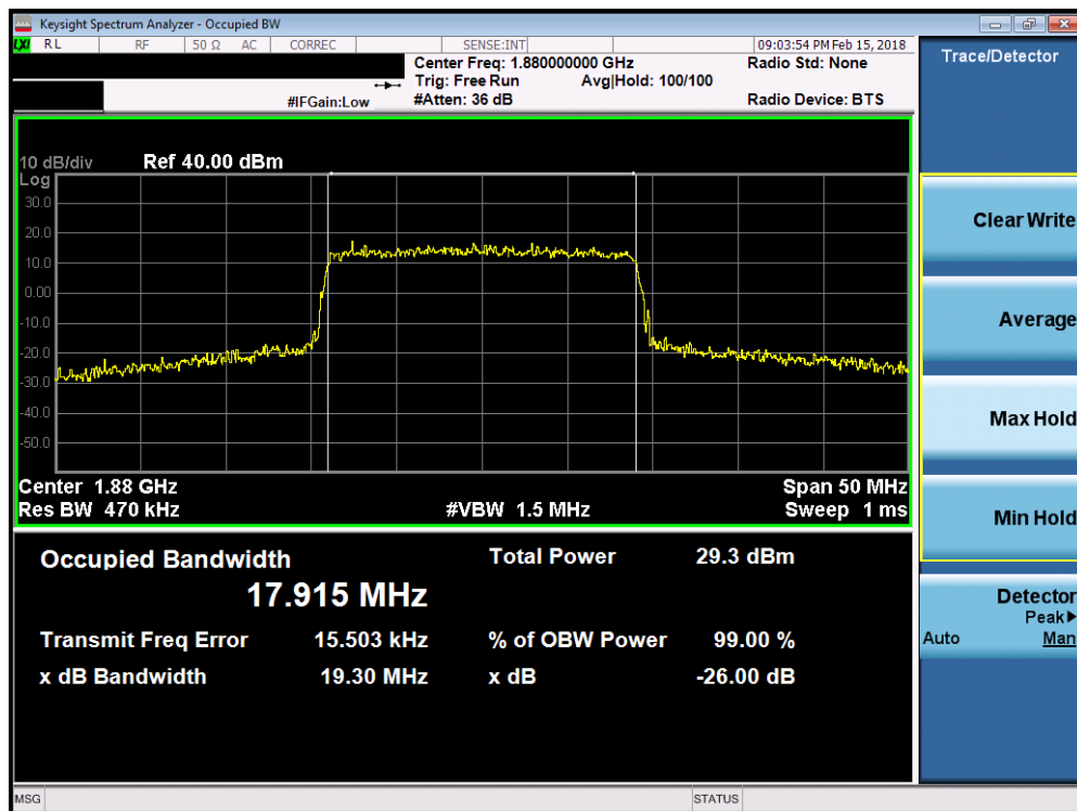
Plot 7-48. Occupied Bandwidth Plot (Band 2 - 20.0MHz 16-QAM - Full RB Configuration)
