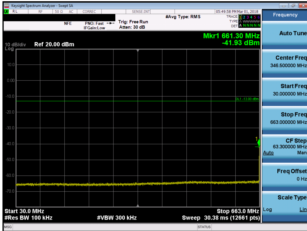
Plot 7-63. Conducted Spurious Plot (Band 71 - 20.0MHz QPSK - RB Size 1, RB Offset 0 - High Channel)
