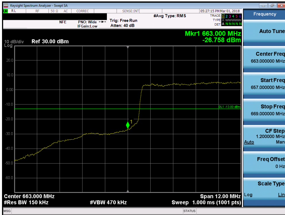
Plot 7-112. Lower Band Edge Plot (Band 71 - 15.0MHz QPSK - Full RB Configuration)
