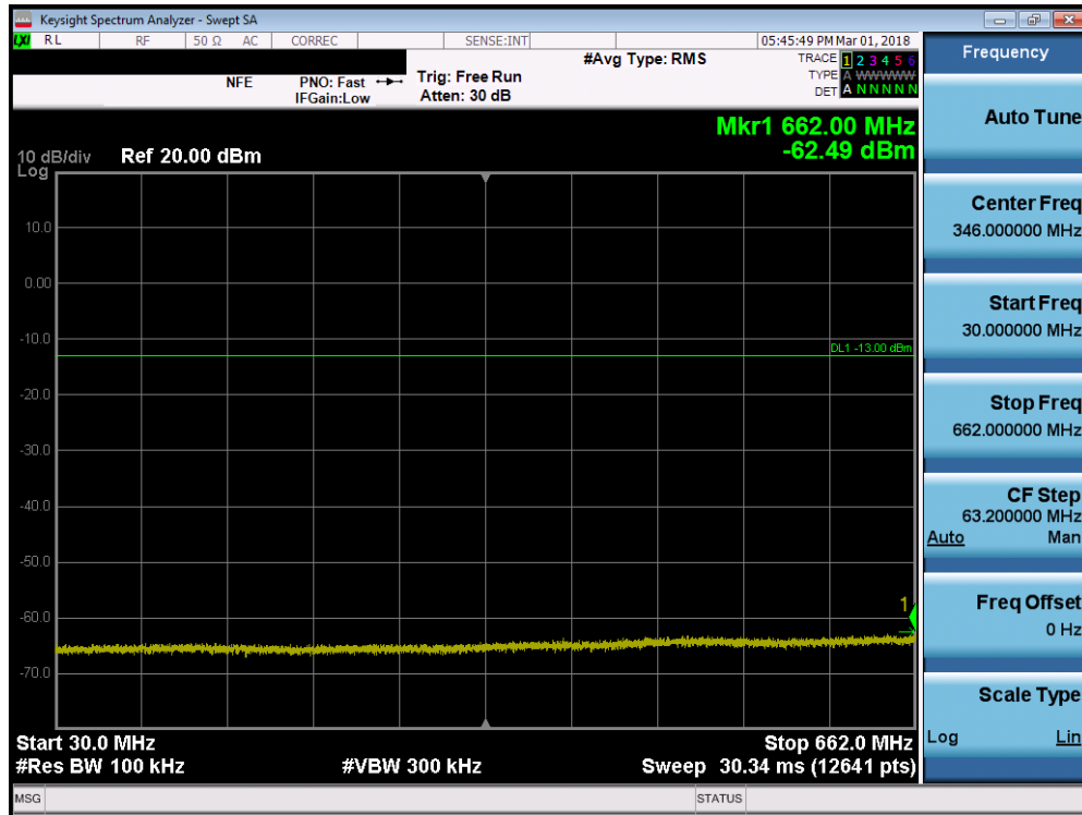
Plot 7-57. Conducted Spurious Plot (Band 71 - 20.0MHz QPSK - RB Size 1, RB Offset 0 - Low Channel)
