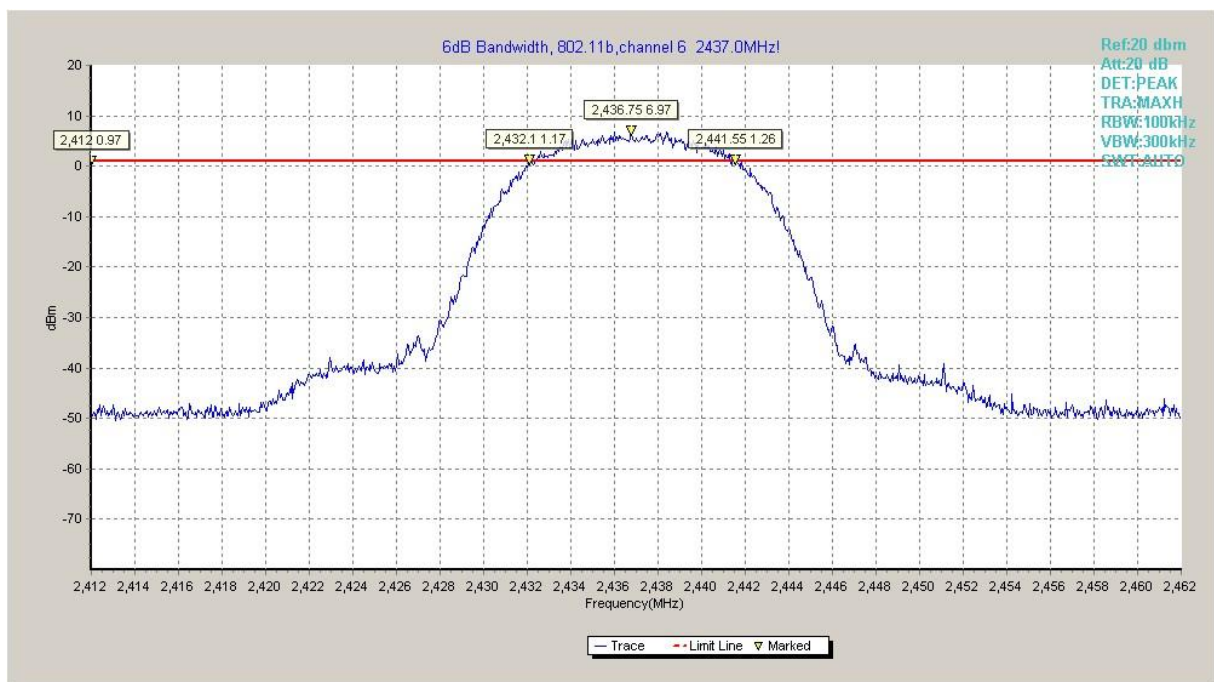
Fig.A.4.2 Occupied 6dB Bandwidth (802.11b, Ch 6)
