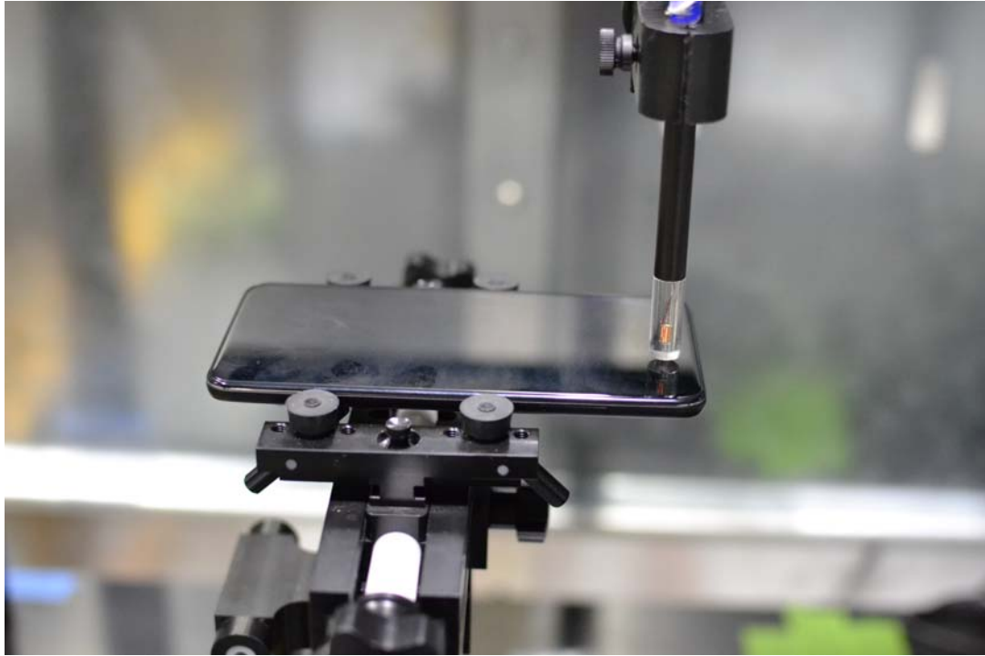
Figure 16-1 Test Setup for Wireless Device
