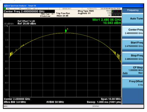
Test Plots (8DPSK) Peak Power (CH.0)
