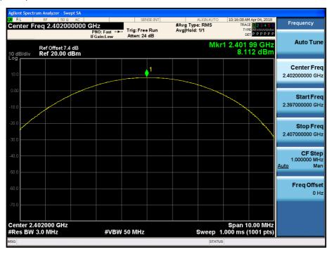
Test Plots (π/4DQPSK) Peak Power (CH.39)
