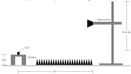
Figure 7-5. Test Instrument & Measurement Setup
