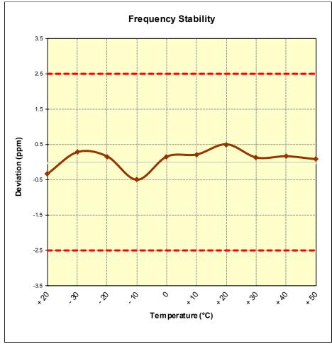
Figure 7-6. CDMA BC10 Frequency Stability Graph (Ch. 476)
