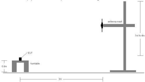
Figure 7-4. Radiated Test Setup <1GHz
