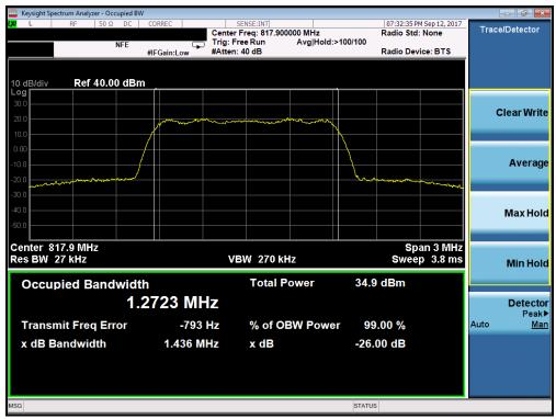
Plot 7-1. CDMA BC10 Occupied Bandwidth Plot (Ch. 476)
