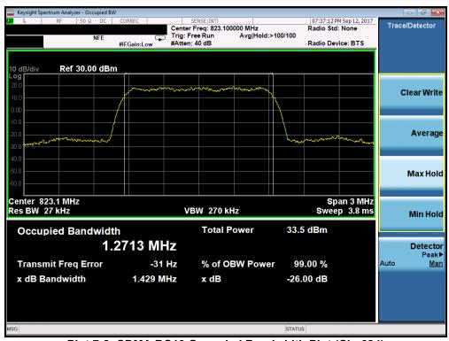
Plot 7-2. CDMA BC10 Occupied Bandwidth Plot (Ch. 684)
