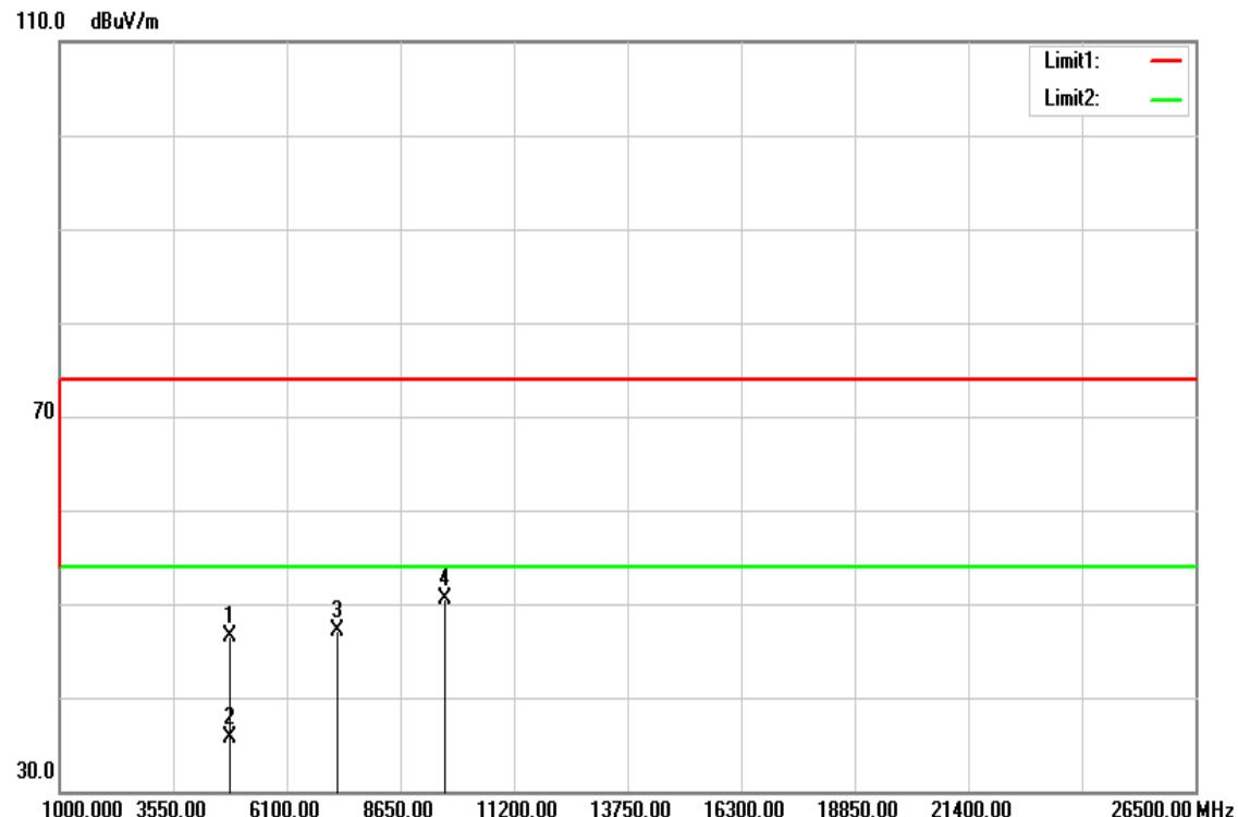
**Operation Mode:** TX / IEEE 802.11g / CH Low**Test Date:** April 28, 2016**Temperature:** 27°C**Tested by:** Dennis Li**Humidity:** 53% RH**Polarity:** Ver. / Hor.
