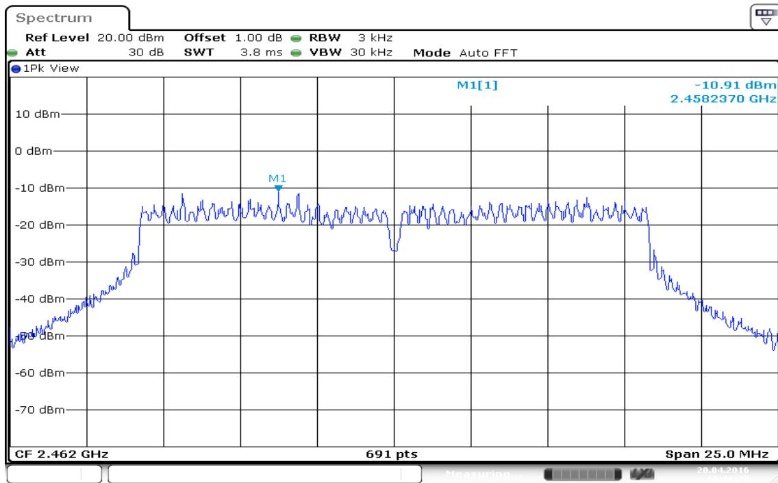
**IEEE 802.11n HT 20 MHz mode****PPSD (CH Low)**
