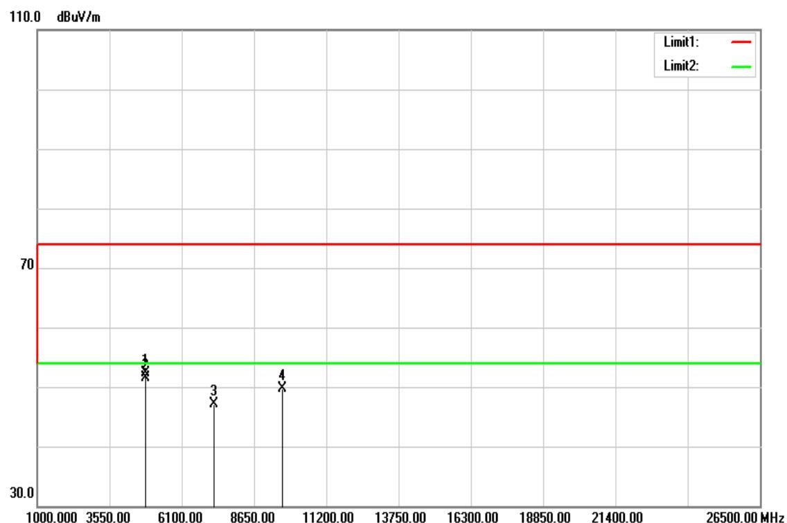
**Above 1 GHz****Operation Mode:** TX / IEEE 802.11b / CH Low**Test Date:** April 28, 2016**Temperature:** 27°C**Tested by:** Dennis Li**Humidity:** 53% RH**Polarity:** Ver. / Hor.
