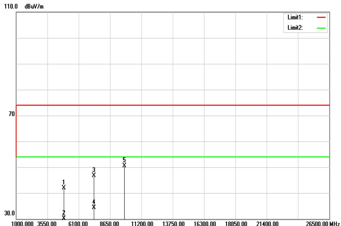
**Operation Mode:** TX / IEEE 802.11n HT 40 MHz mode / CH High **Test Date:** April 28, 2016
