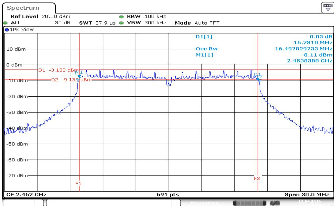
**IEEE 802.11n HT 20 MHz mode****99% Bandwidth (CH Low)**
