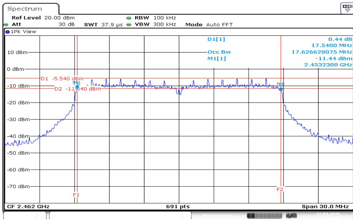
**IEEE 802.11n HT 40 MHz mode****6dB Bandwidth (CH Low)**
