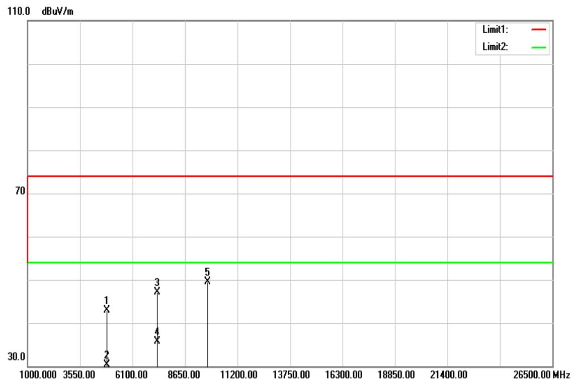
**Operation Mode:** TX / IEEE 802.11n HT 20 MHz mode / CH Mid**Test Date:** April 28, 2016**Temperature:** 27°C**Tested by:** Dennis Li**Humidity:** 53% RH**Polarity:** Ver. / Hor.
