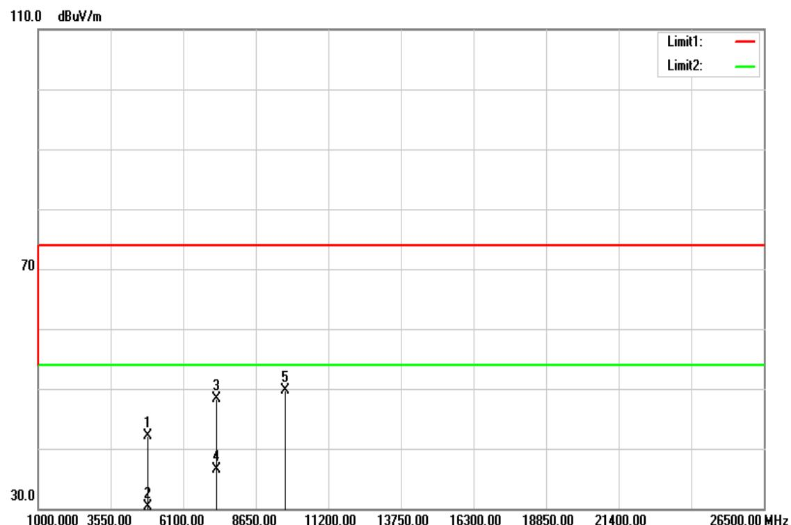
**Operation Mode:** TX / IEEE 802.11n HT 40 MHz mode / CH Low **Test Date:** April 28, 2016
