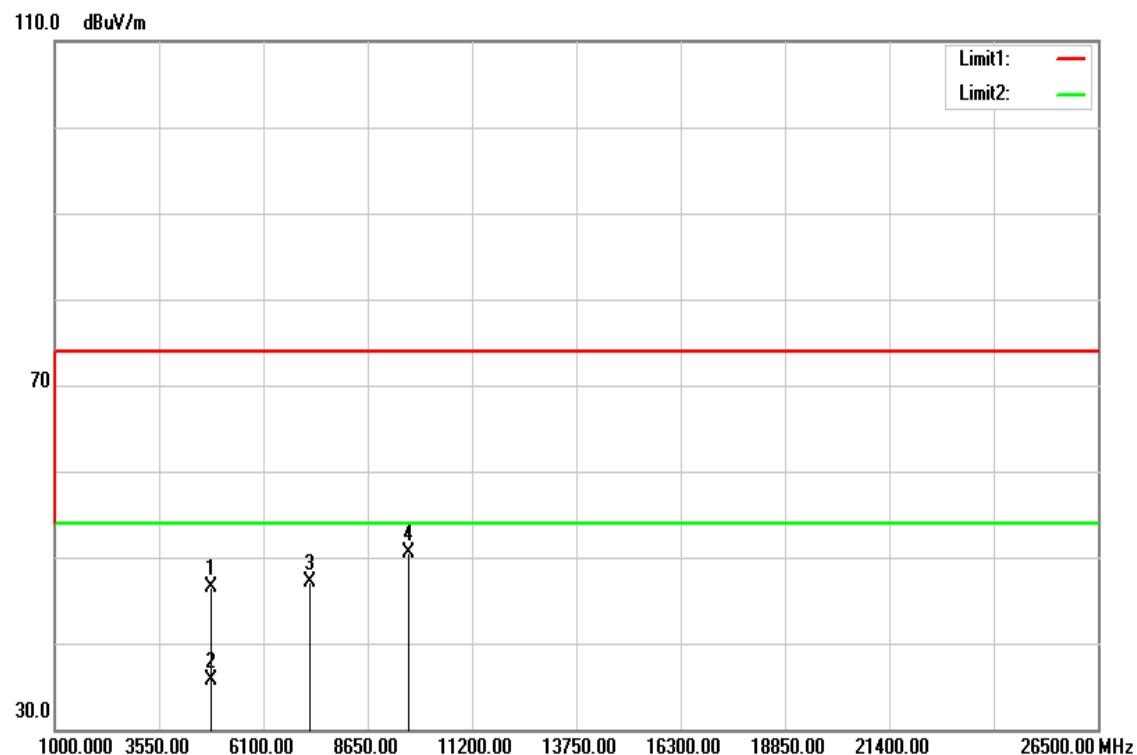
**Operation Mode:** TX / IEEE 802.11g / CH Mid**Test Date:** April 28, 2016**Temperature:** 27°C**Tested by:** Dennis Li**Humidity:** 53% RH**Polarity:** Ver. / Hor.
