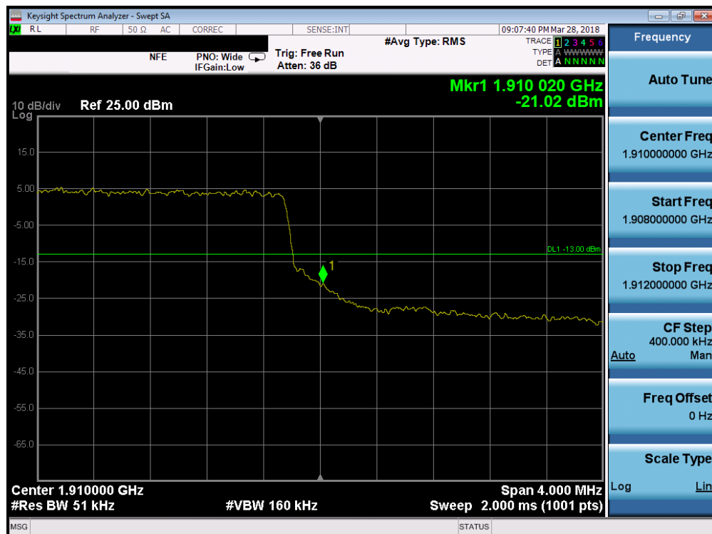
Plot 7-134. Upper Band Edge Plot (Band 2 - 5.0MHz QPSK - Full RB Configuration)
