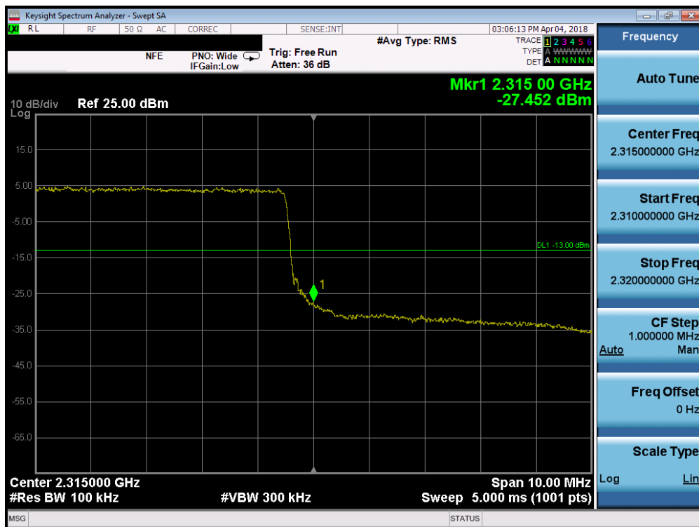
Plot 7-154. Upper Band Edge Plot (Band 30 - 10.0MHz QPSK - Full RB Configuration)
