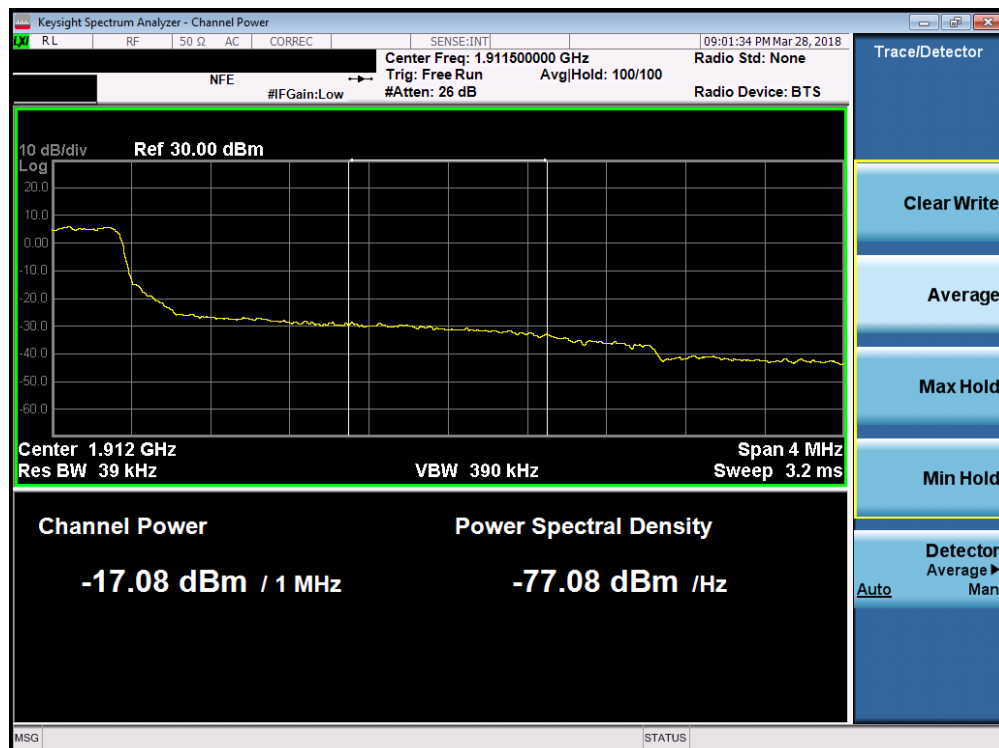
Plot 7-131. Upper Extended Band Edge Plot (Band 2 - 3.0MHz QPSK - Full RB Configuration)
