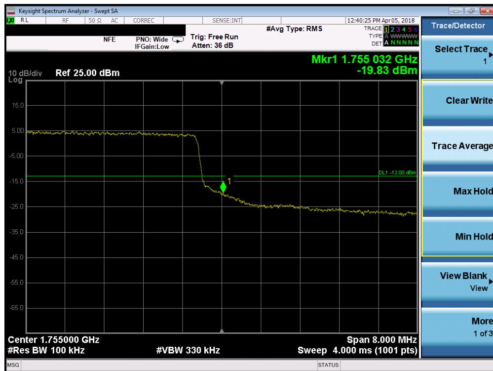
Plot 7-114. Upper Band Edge Plot (Band 4 - 10.0MHz QPSK - Full RB Configuration)
