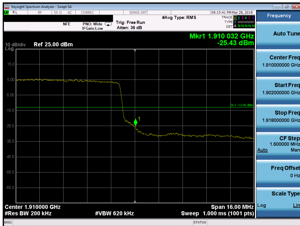
Plot 7-146. Upper Band Edge Plot (Band 2 - 20.0MHz QPSK - Full RB Configuration)
