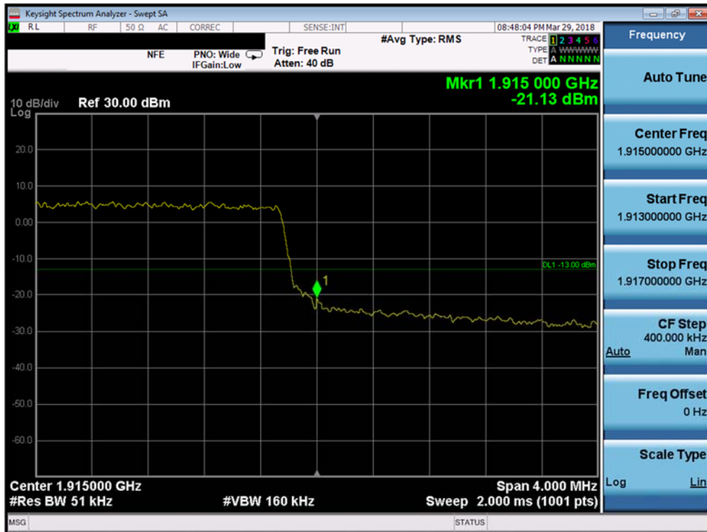
Plot 7-189. Upper Band Edge Plot (Band 25 - 5.0MHz QPSK - Full RB Configuration)
