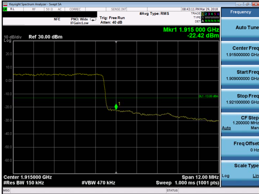
Plot 7-201. Upper Band Edge Plot (Band 25 - 15.0MHz QPSK - Full RB Configuration)
