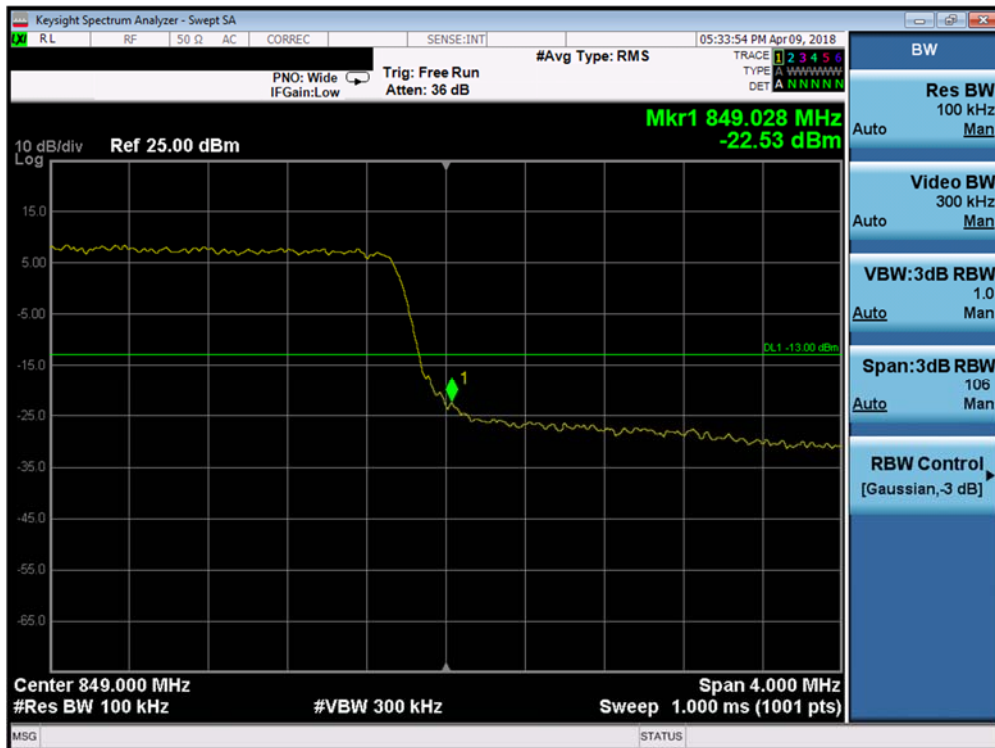
Plot 7-144. Upper Band Edge Plot (Band 26/5 - 5.0MHz QPSK - Full RB Configuration)
