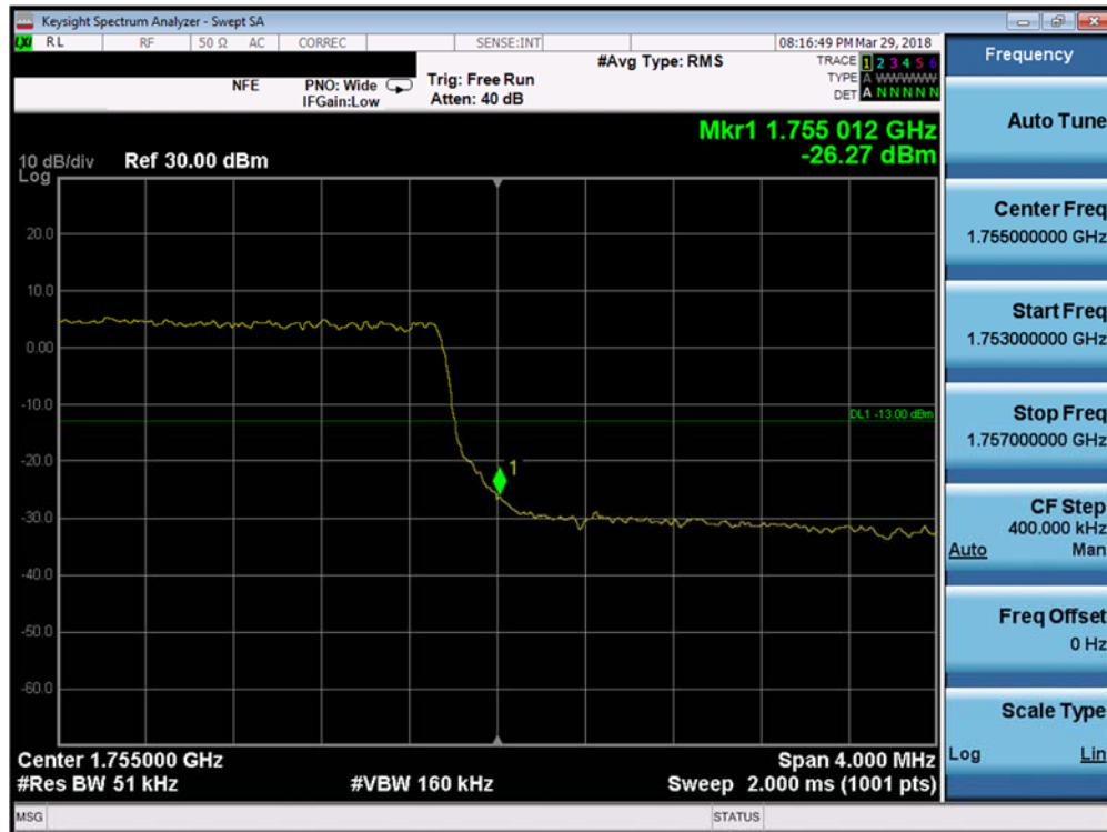
Plot 7-159. Upper Band Edge Plot (Band 4 - 5.0MHz QPSK - Full RB Configuration)
