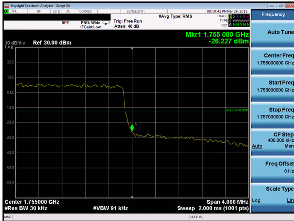
Plot 7-155. Upper Band Edge Plot (Band 4 - 3.0MHz QPSK - Full RB Configuration)
