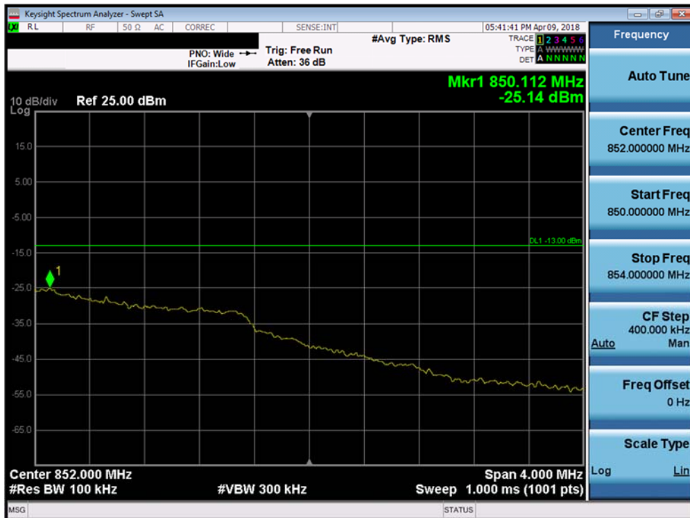
Plot 7-142. Upper Extended Band Edge Plot (Band 26/5 - 3.0MHz QPSK - Full RB Configuration)
