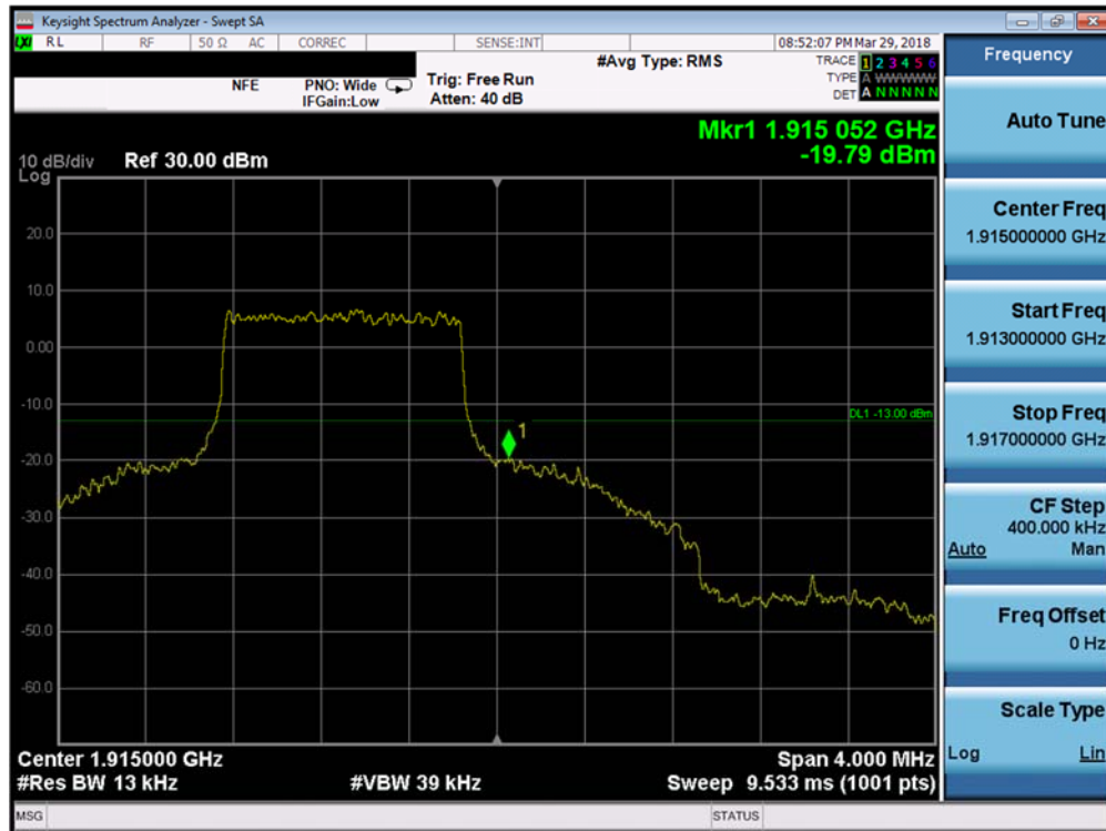
Plot 7-177. Upper Band Edge Plot (Band 25 - 1.4MHz QPSK - Full RB Configuration)
