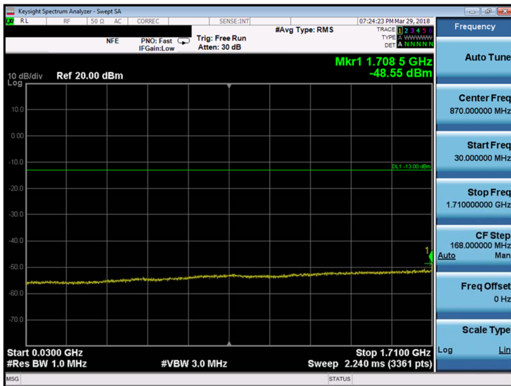
Plot 7-93. Conducted Spurious Plot (Band 4 - 20.0MHz QPSK - RB Size 1, RB Offset 0 - Mid Channel)
