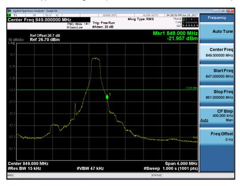
BAND 5. Upper Band Edge Plot (1.4M BW Ch.20643 QPSK\_RB6\_Offset 0)
