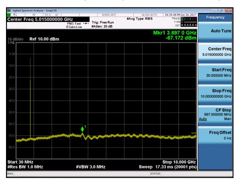
BAND 5. Conducted Spurious Plot (20525ch\_5MHz\_QPSK\_RB 1\_0)
