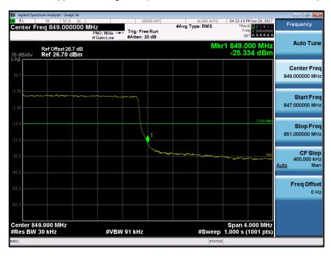
BAND 5. Upper Extended Band Edge Plot (3M BW Ch.20635 QPSK\_RB15\_0)
