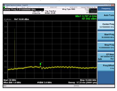
BAND 5. Conducted Spurious Plot (20525ch\_1.4MHz\_QPSK\_RB 1\_0)
