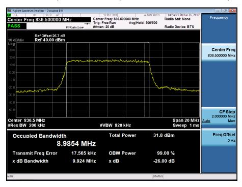
BAND 5. Occupied Bandwidth Plot (10M BW Ch.20525 16QAM\_RB50\_0)
