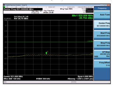
BAND 5. Lower Band Edge Plot (10M BW Ch.20450 QPSK\_RB1\_Offset 0)
