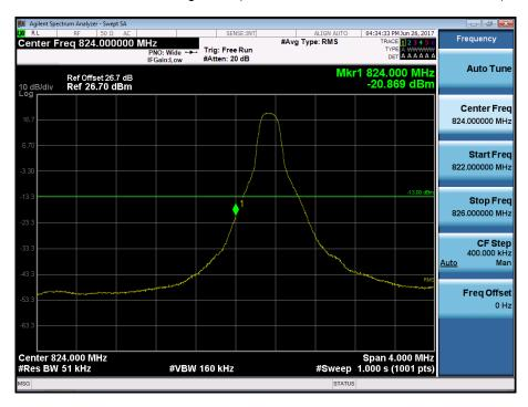
BAND 5. Lower Band Edge Plot (5M BW Ch.20425 QPSK\_RB25\_Offset 0)
