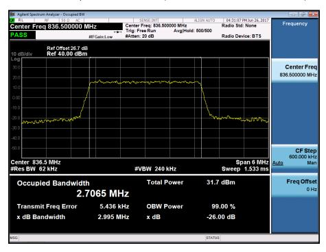
BAND 5. Occupied Bandwidth Plot (3M BW Ch.20525 16QAM\_RB15\_0)
