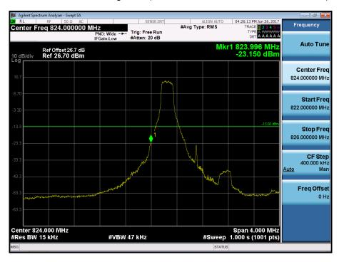
BAND 5. Lower Band Edge Plot (1.4M BW Ch.20407 QPSK\_RB6\_Offset 0)
