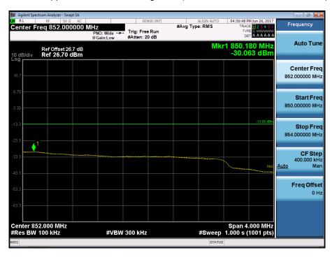
BAND 5. Upper Band Edge Plot (10M BW Ch.20600 QPSK\_RB1\_Offset 49)
