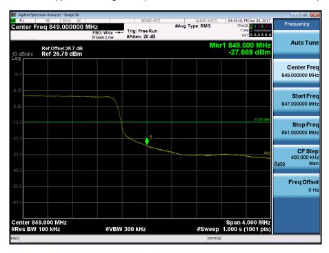
BAND 5. Upper Extended Band Edge Plot (10M BW Ch.20600 QPSK\_RB50\_0)
