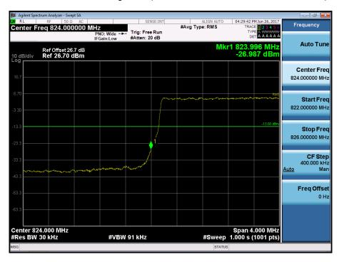
BAND 5. Lower Extended Band Edge Plot (3M BW Ch.20415 QPSK\_RB15\_0)
