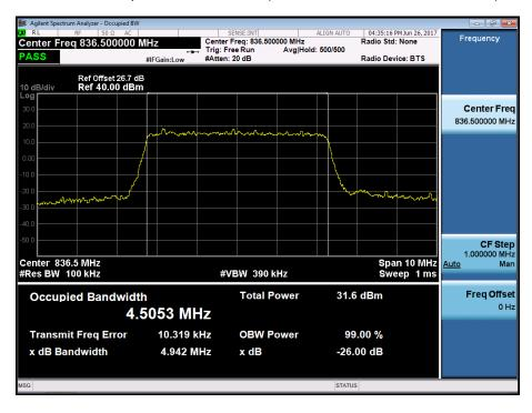
BAND 5. Occupied Bandwidth Plot (5M BW Ch.20525 16QAM\_RB25\_0)
