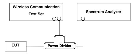
(Configuration of conducted Emission measurement)
