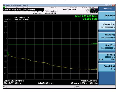
BAND 5. Upper Band Edge Plot (3M BW Ch.20635 QPSK\_RB1\_Offset 14)
