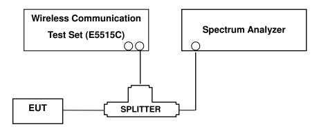
(Configuration of conducted Emission measurement)
