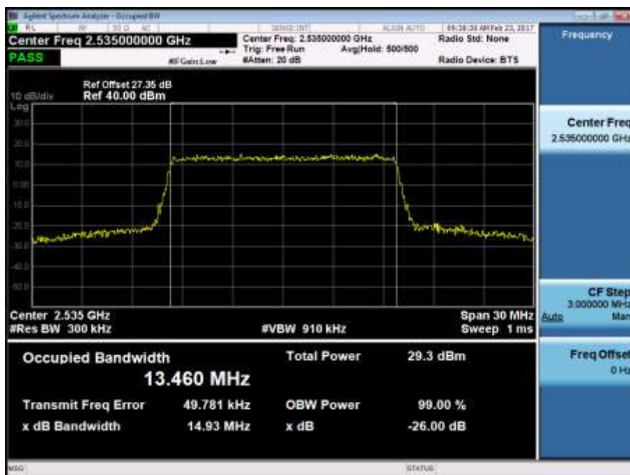
BAND7. Occupied Bandwidth Plot (15MHz Ch.21100 16-QAM RB 75)
