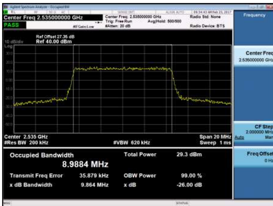
BAND7. Occupied Bandwidth Plot (10MHz Ch.21100 16-QAM RB 50)
