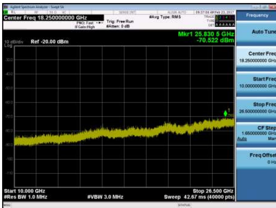
BAND7. Conducted Spurious Plot 2 (10MHz Ch.21400 QPSK RB 1, Offset 0)
