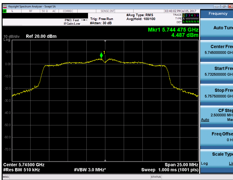
Plot 7-144. Power Spectral Density Plot (802.11a (UNII Band 3) – Ch. 149)
