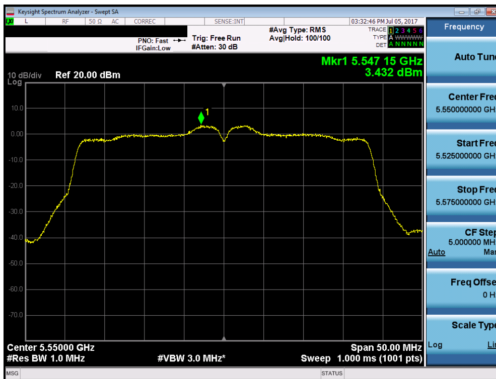
Plot 7-140. Power Spectral Density Plot (40MHz BW 802.11n (UNII Band 2C) – Ch. 110)
