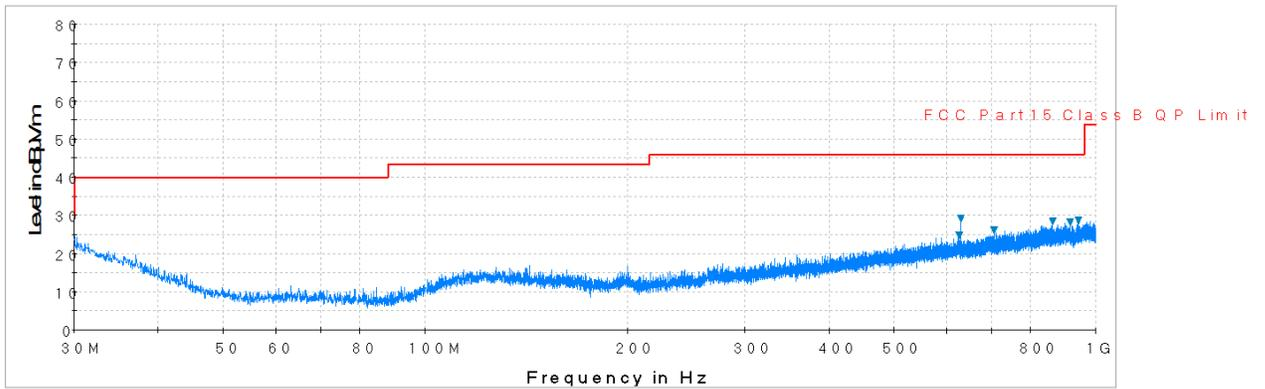
Plot 7-52. Radiated Spurious Plot below 1GHz (Pol. V)
