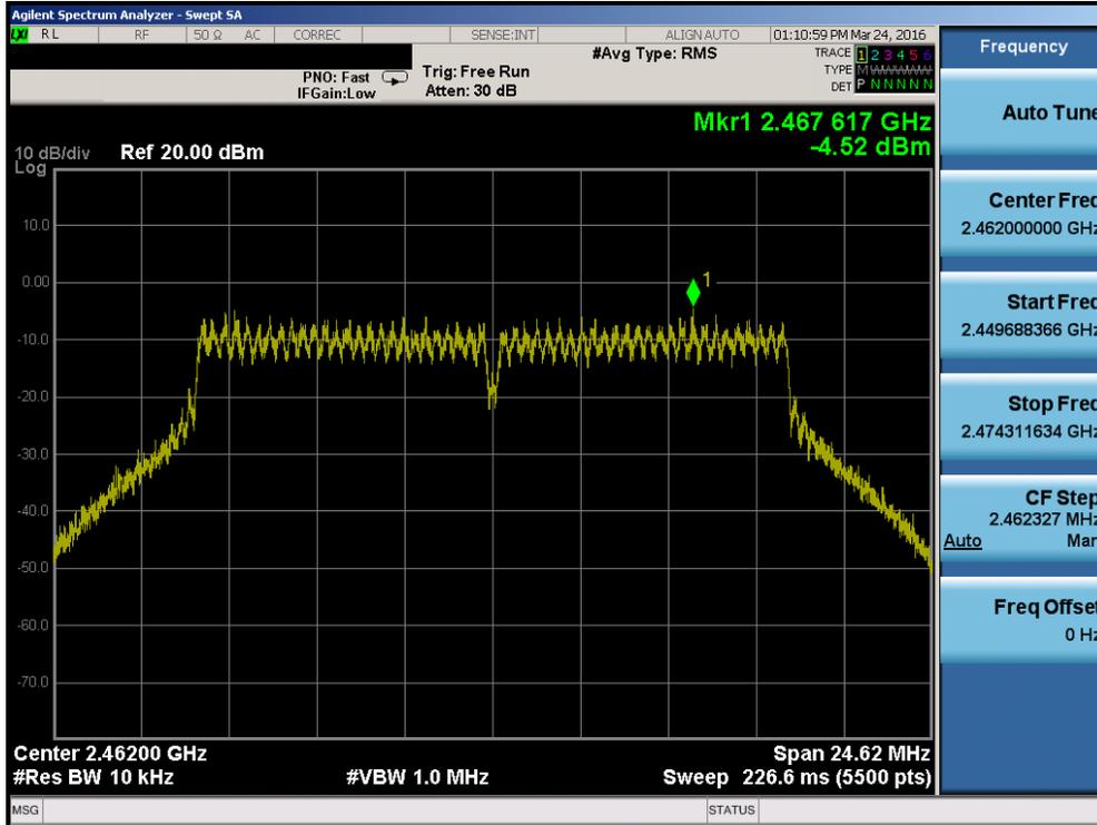
Plot 7-15. Power Spectral Density Plot (802.11g – Ch. 11)
