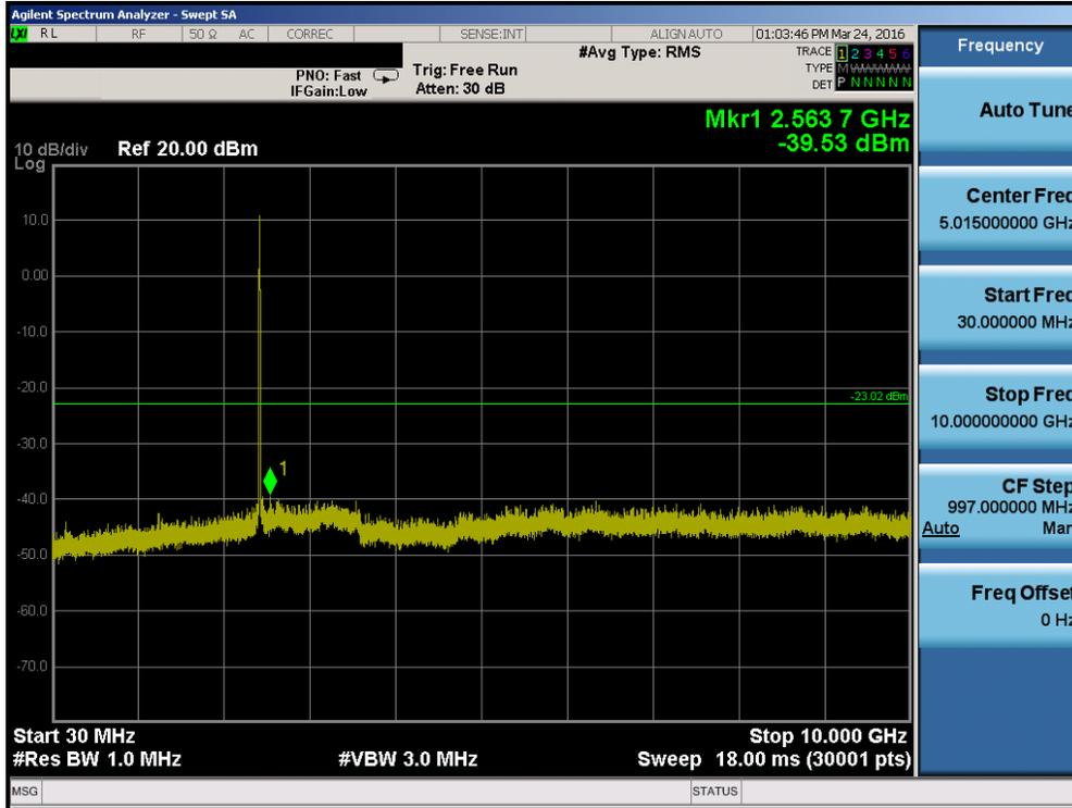
Plot 7-31. Conducted Spurious Plot (802.11b – Ch. 6)
