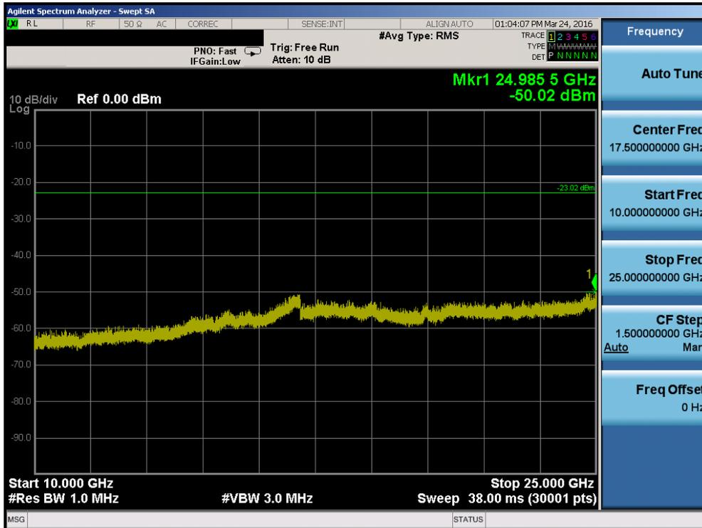
Plot 7-32. Conducted Spurious Plot (802.11b – Ch. 6)
