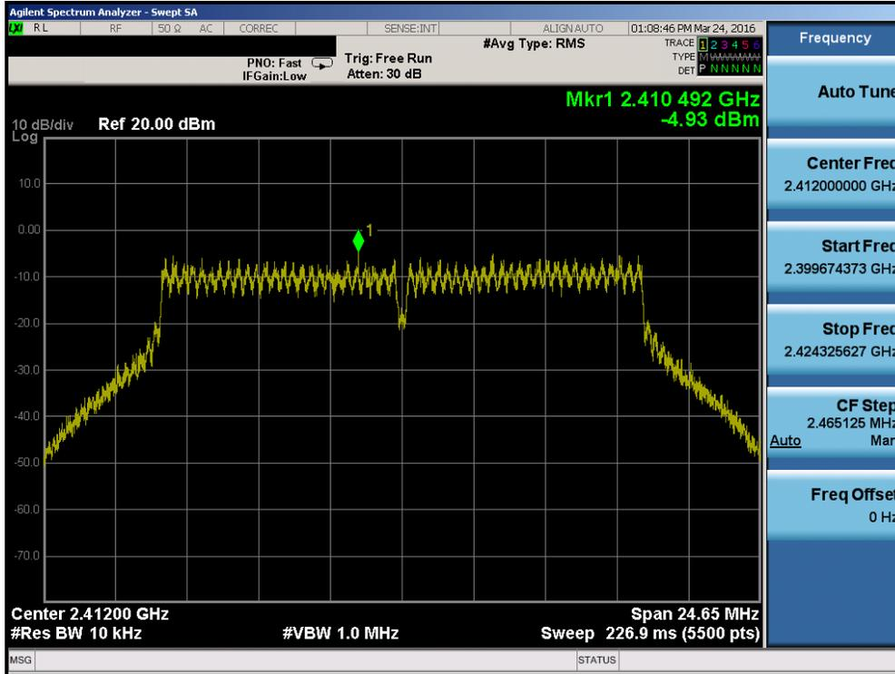
Plot 7-13. Power Spectral Density Plot (802.11g – Ch. 1)
