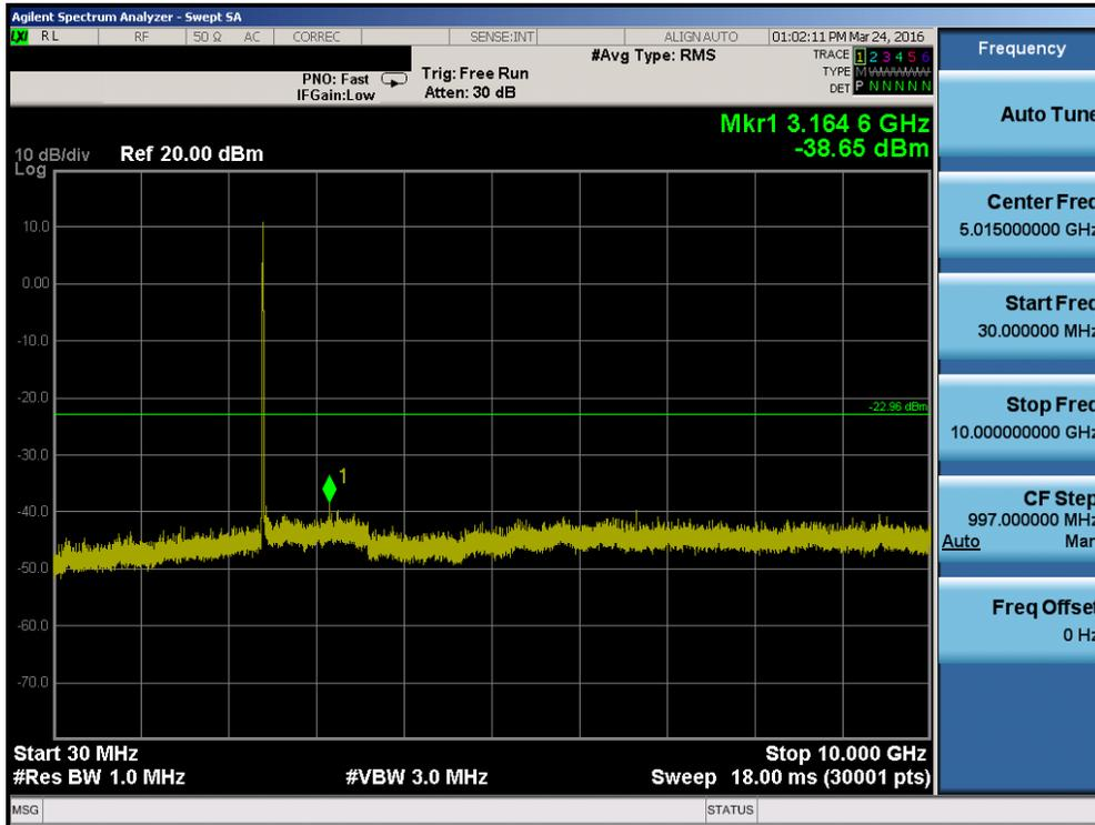
Plot 7-29. Conducted Spurious Plot (802.11b – Ch. 1)
