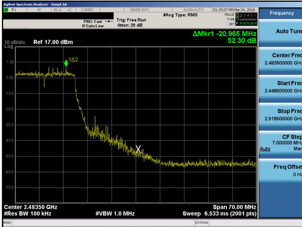
Plot 7-27. Band Edge Plot (802.11n (2.4GHz) – Ch. 10)
