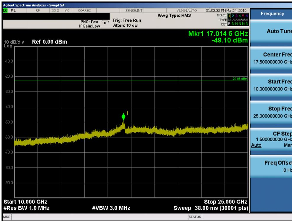
Plot 7-30. Conducted Spurious Plot (802.11b – Ch. 1)
