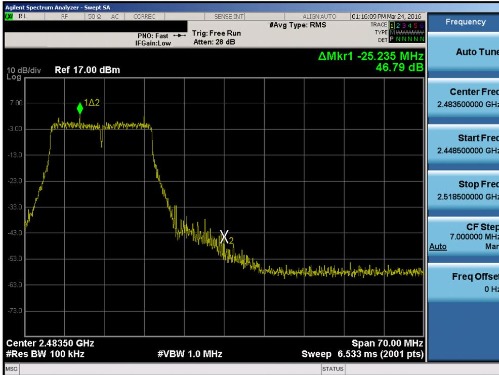
Plot 7-28. Band Edge Plot (802.11n (2.4GHz) – Ch. 11)
