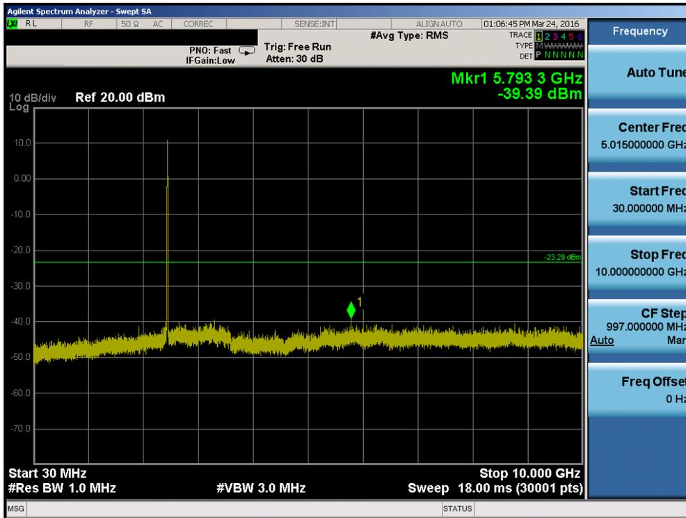
Plot 7-33. Conducted Spurious Plot (802.11b – Ch. 11)
