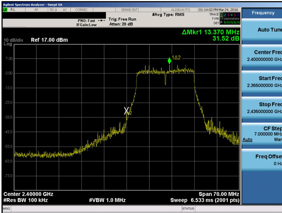
Plot 7-25. Band Edge Plot (802.11n (2.4GHz) – Ch. 1)
