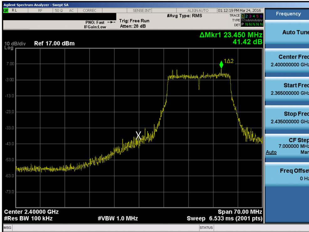
Plot 7-26. Band Edge Plot (802.11n (2.4GHz) – Ch. 2)
