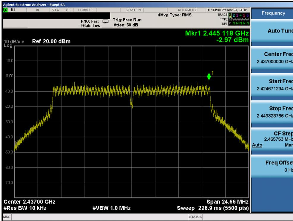
Plot 7-14. Power Spectral Density Plot (802.11g – Ch. 6)
