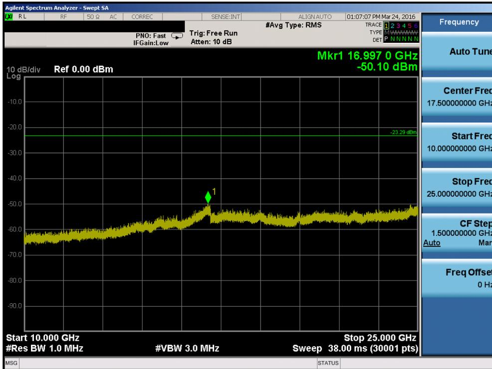
Plot 7-34. Conducted Spurious Plot (802.11b – Ch. 11)
