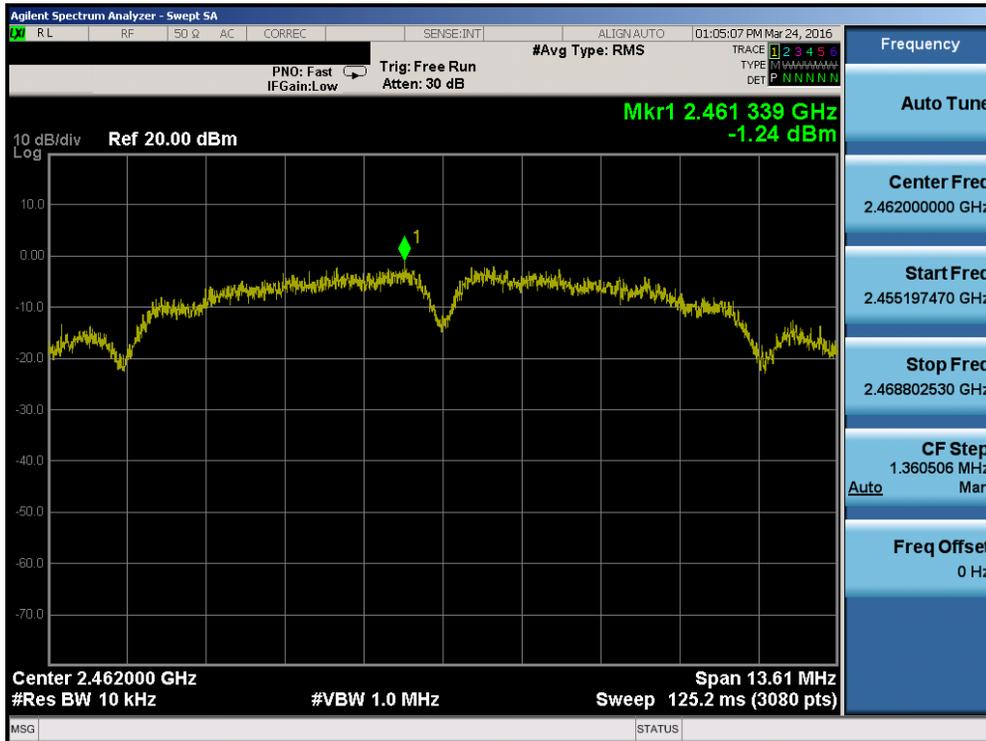
Plot 7-12. Power Spectral Density Plot (802.11b – Ch. 11)
