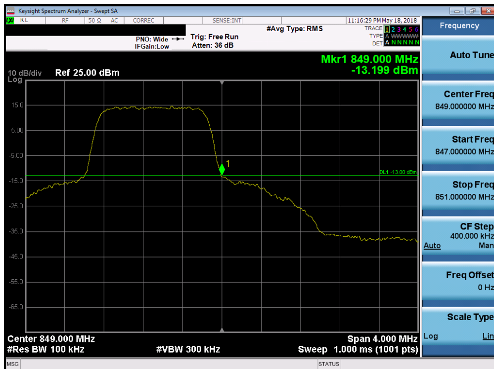
Plot 7-132. Upper Band Edge Plot (Band 5 - 1.4MHz QPSK - Full RB Configuration)
