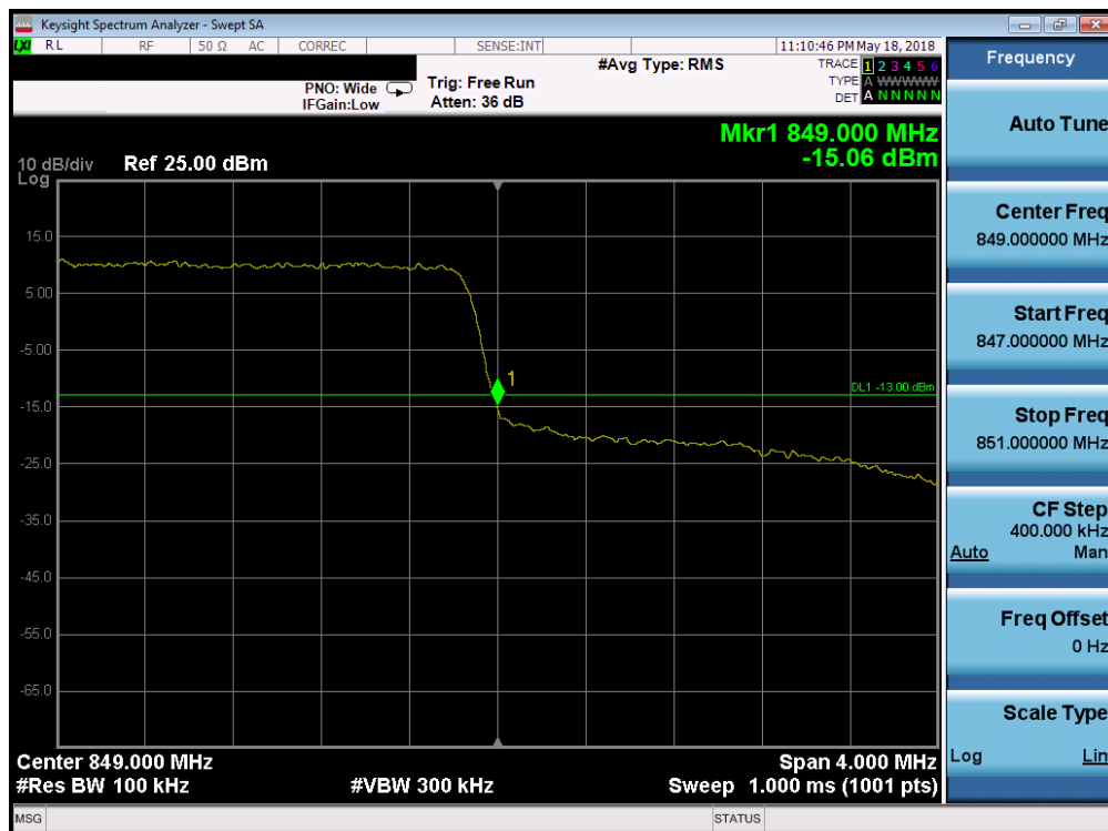
Plot 7-134. Upper Band Edge Plot (Band 5 - 3.0MHz QPSK - Full RB Configuration)
