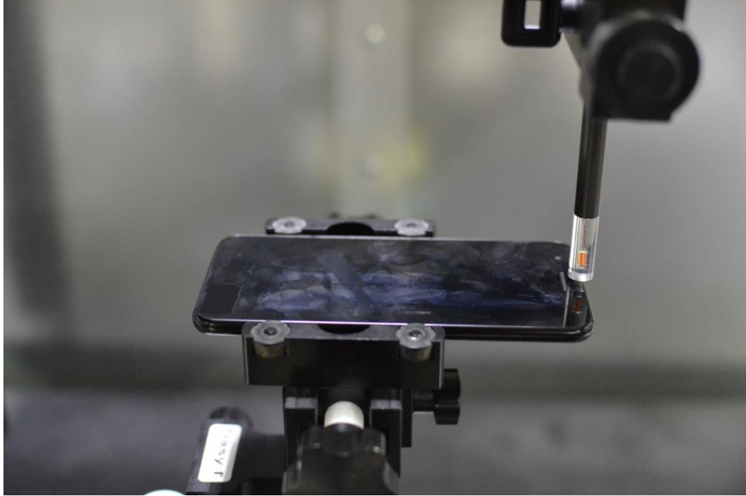
Figure 16-1 Test Setup for Wireless Device
