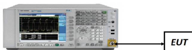
Figure 7-4. Test Instrument & Measurement Setup
