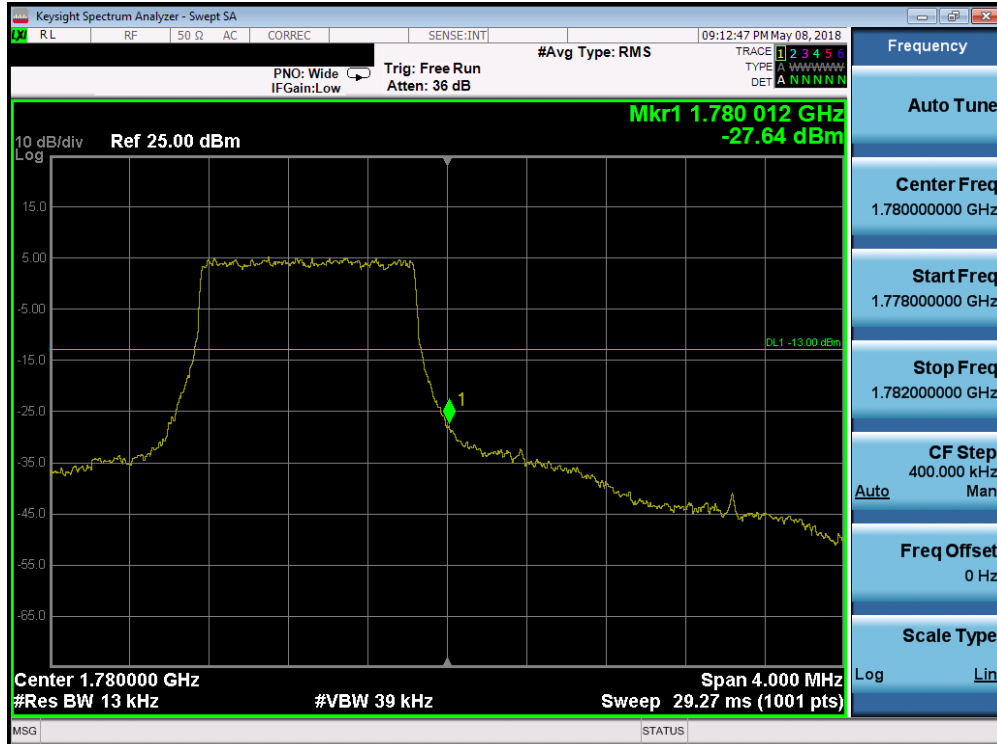
Plot 7-122. Upper Band Edge Plot (Band 66 - 1.4MHz QPSK - Full RB Configuration)
