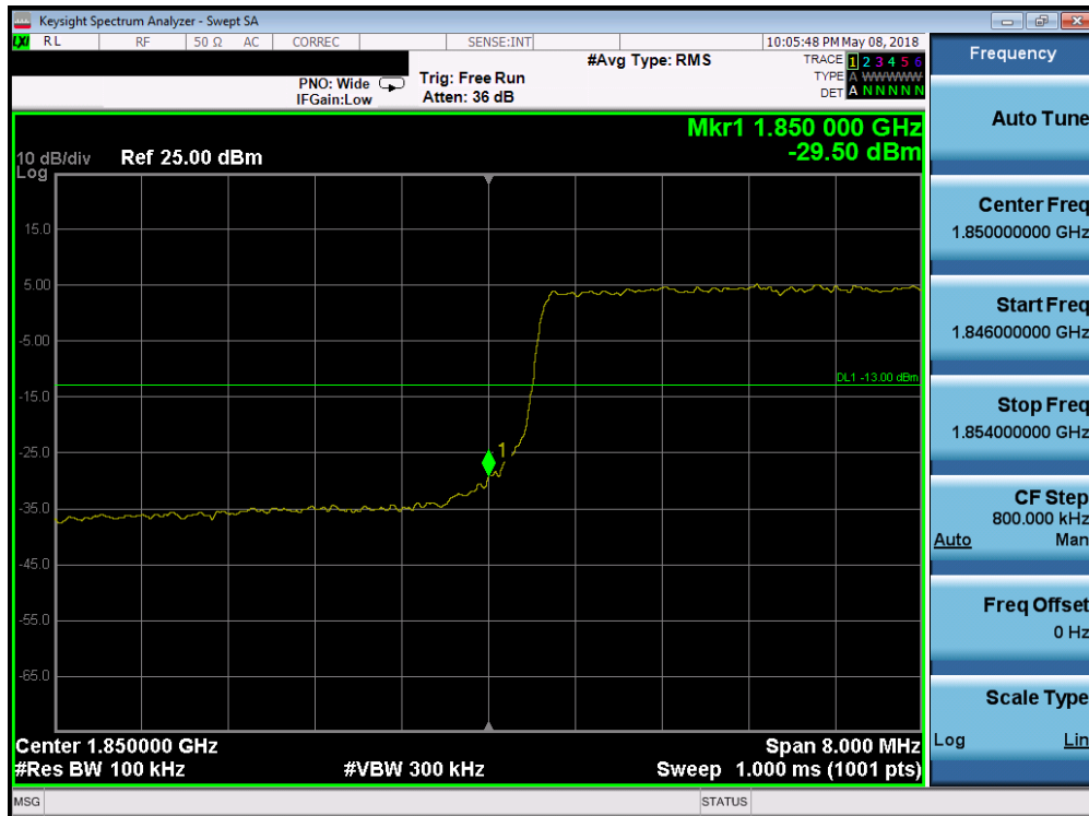
Plot 7-166. Lower Band Edge Plot (Band 2 - 10.0MHz QPSK - Full RB Configuration)
