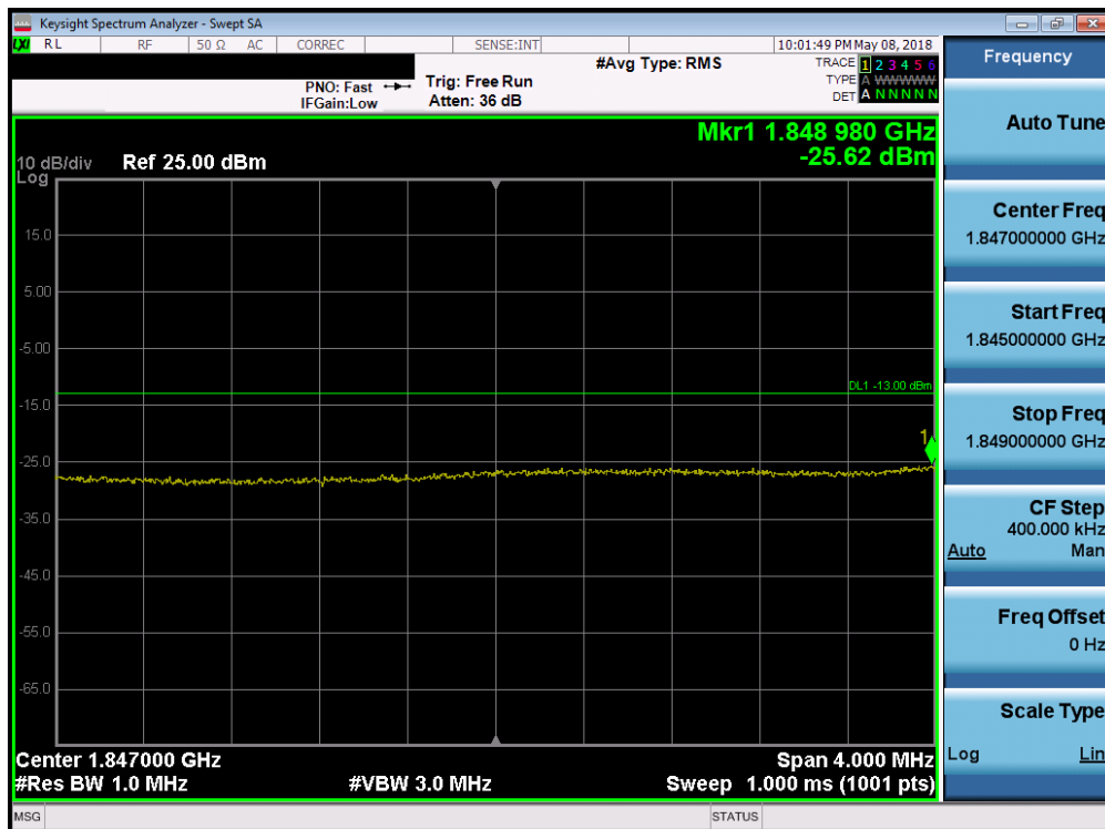
Plot 7-171. Lower Extended Band Edge Plot (Band 2 - 15.0MHz QPSK - Full RB Configuration)
