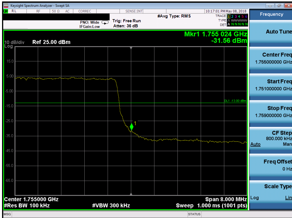
Plot 7-138. Upper Band Edge Plot (Band 4 - 10.0MHz QPSK - Full RB Configuration)
