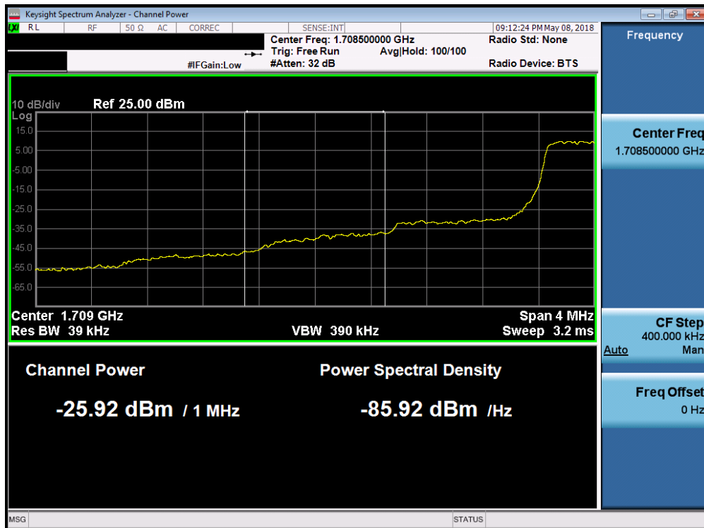
Plot 7-119. Lower Extended Band Edge Plot (Band 66/4 - 1.4MHz QPSK - Full RB Configuration)
