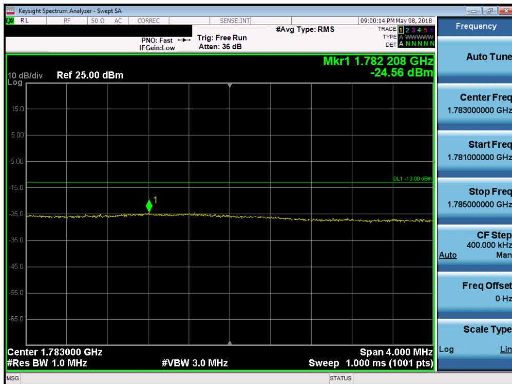
Plot 7-147. Upper Extended Band Edge Plot (Band 66 - 15.0MHz QPSK - Full RB Configuration)
