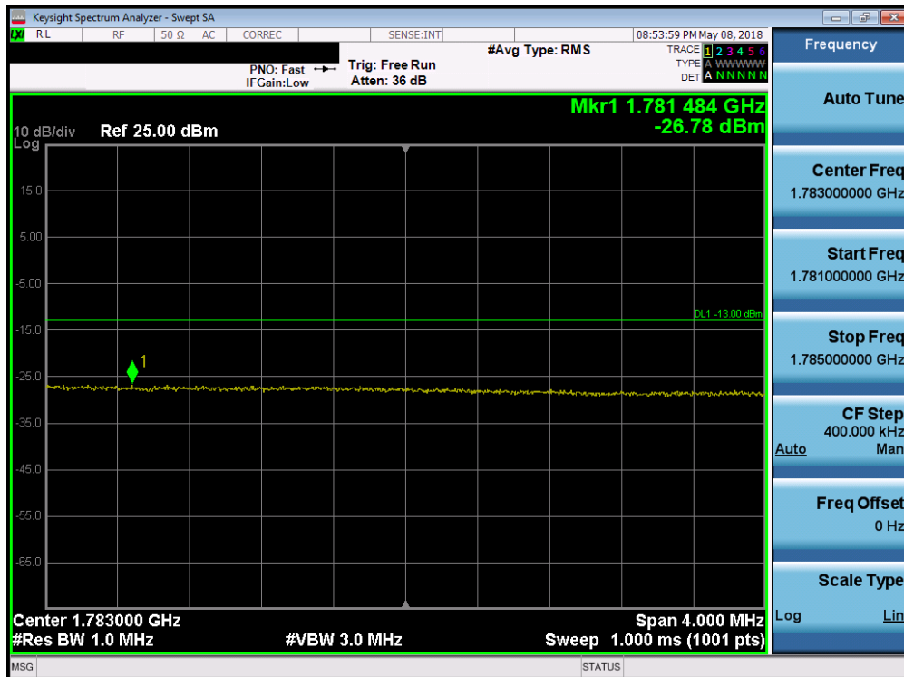
Plot 7-153. Upper Extended Band Edge Plot (Band 66 - 20.0MHz QPSK - Full RB Configuration)
