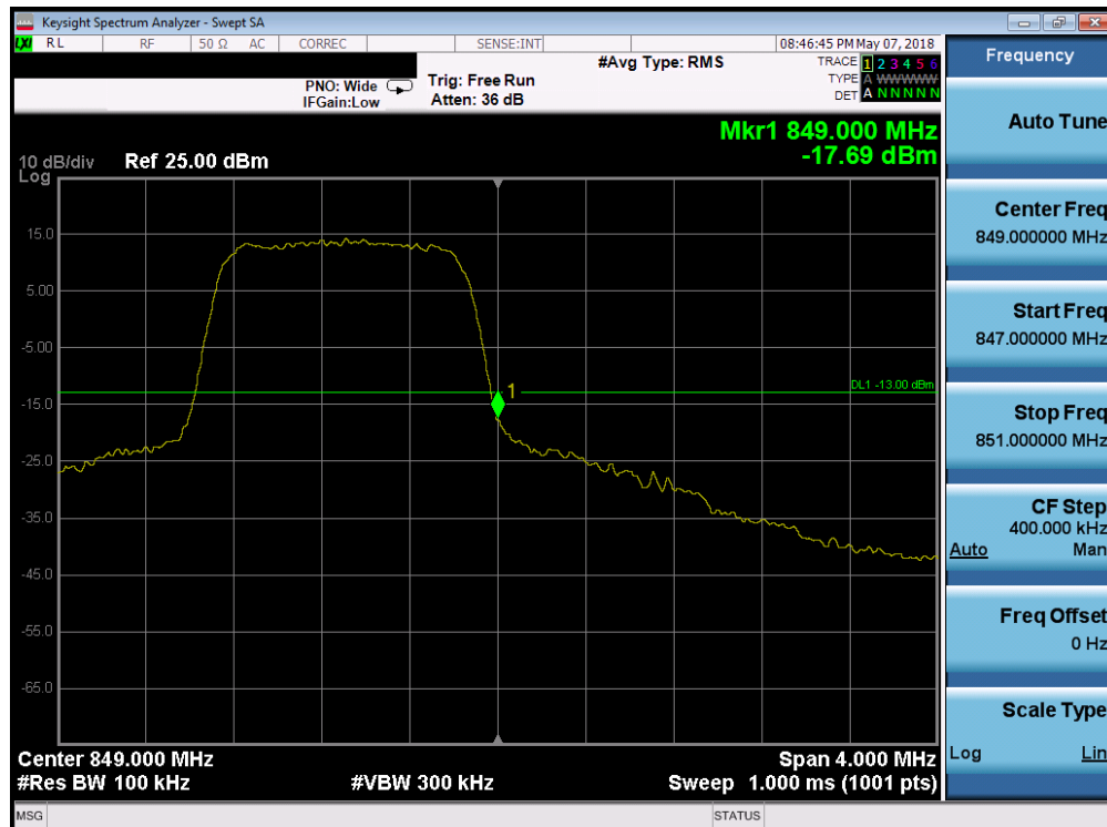
Plot 7-111. Upper Band Edge Plot (Band 5 - 1.4MHz QPSK - Full RB Configuration)
