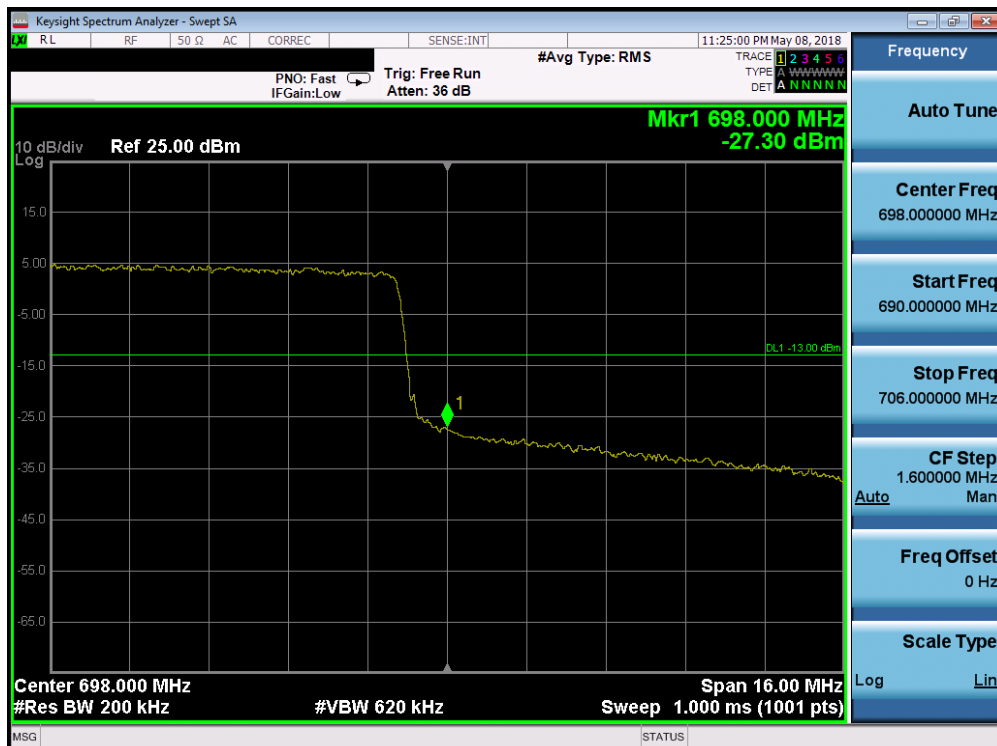
Plot 7-101. Upper Band Edge Plot (Band 71 - 20.0MHz QPSK - Full RB Configuration)
