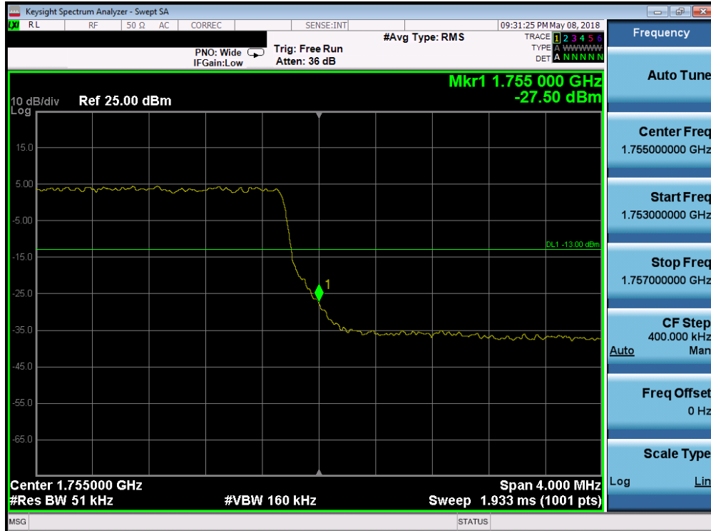
Plot 7-132. Upper Band Edge Plot (Band 4 - 5.0MHz QPSK - Full RB Configuration)
