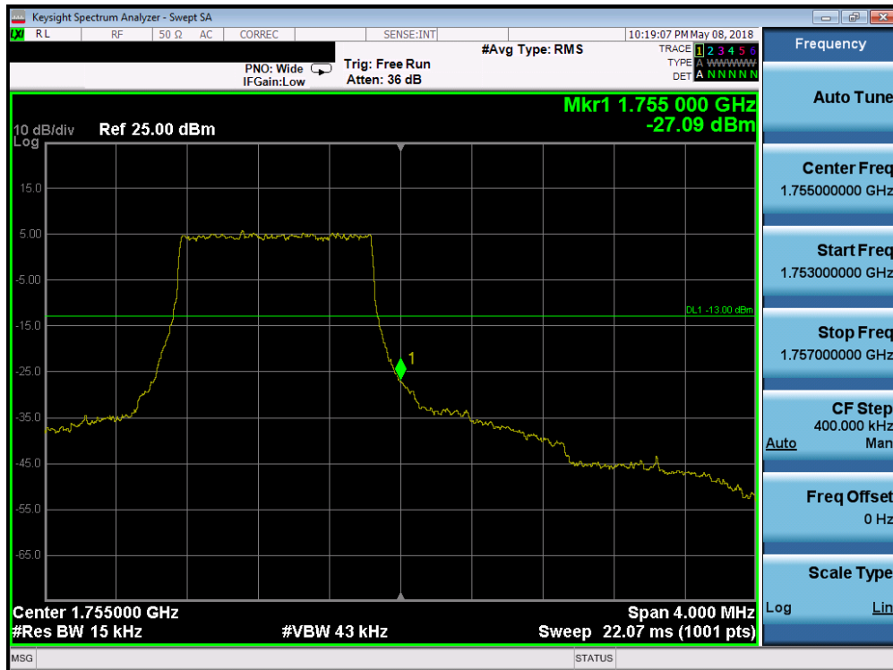
Plot 7-120. Upper Band Edge Plot (Band 4 - 1.4MHz QPSK - Full RB Configuration)
