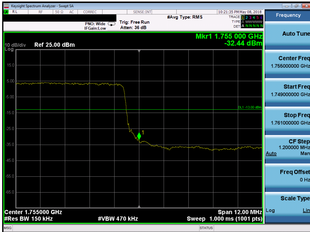
Plot 7-144. Upper Band Edge Plot (Band 4 - 15.0MHz QPSK - Full RB Configuration)
