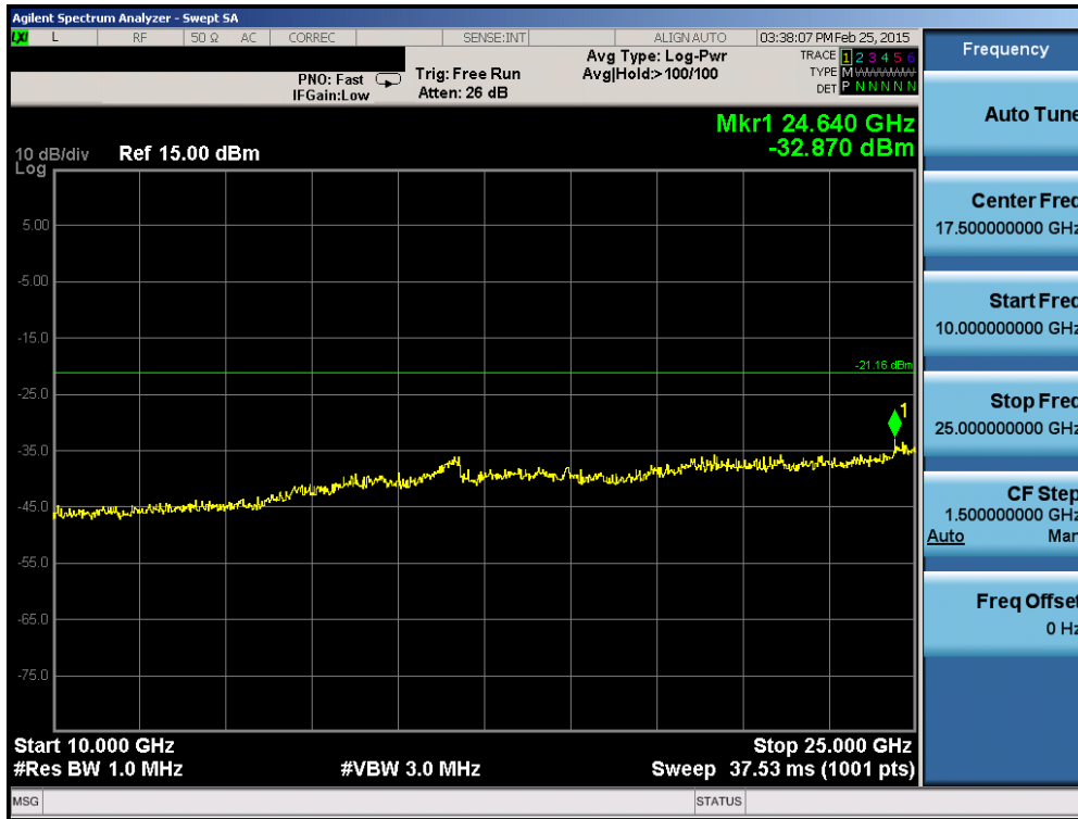
Plot 6-13. Conducted Spurious Plot (Bluetooth (LE) – Ch. 0)
