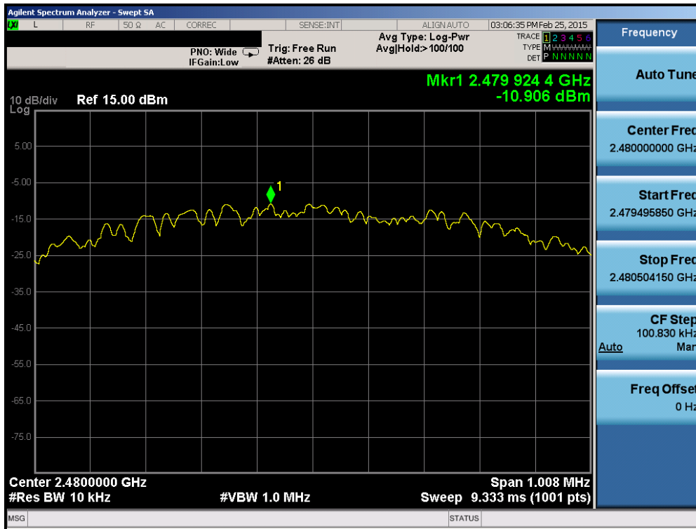
Plot 6-9. Power Spectral Density Plot (Bluetooth (LE) – Ch. 39)
