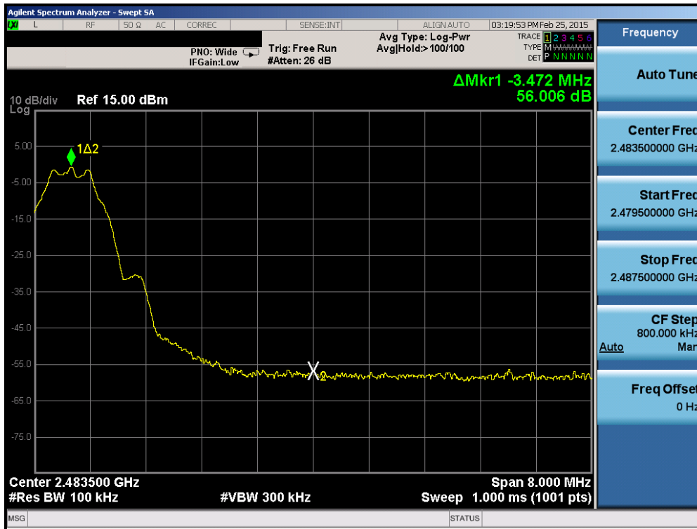
Plot 6-11. Band Edge Plot (Bluetooth (LE) – Ch. 39)
