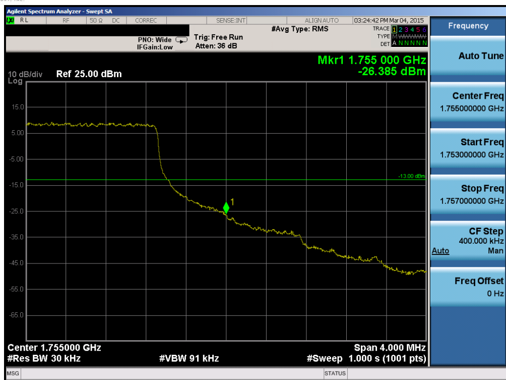
Plot 6-74. Upper Band Edge Plot (Band 4 - 3.0MHz QPSK - RB Size 15)
