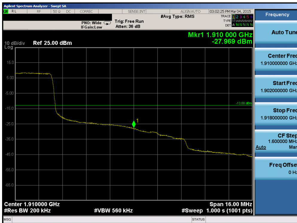
Plot 6-114. Upper Band Edge Plot (Band 2 – 20.0MHz QPSK – RB Size 100)
