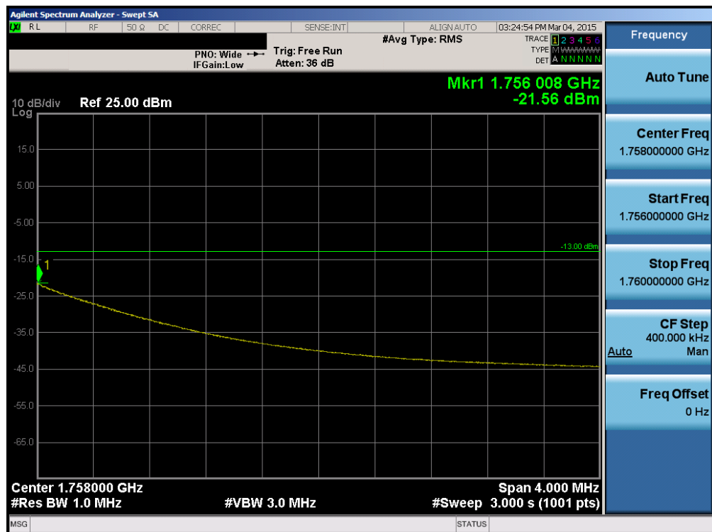
Plot 6-75. Upper Extended Band Edge Plot (Band 4 - 3.0MHz QPSK - RB Size 15)
