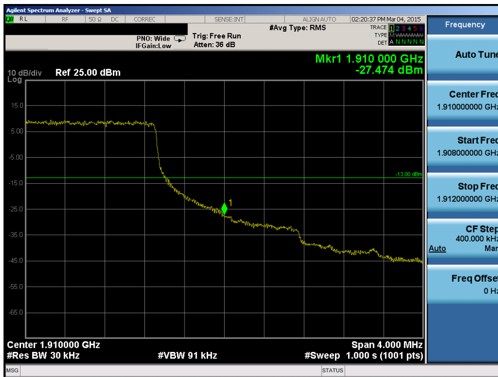
Plot 6-98. Upper Band Edge Plot (Band 2 - 3.0MHz QPSK - RB Size 15)
