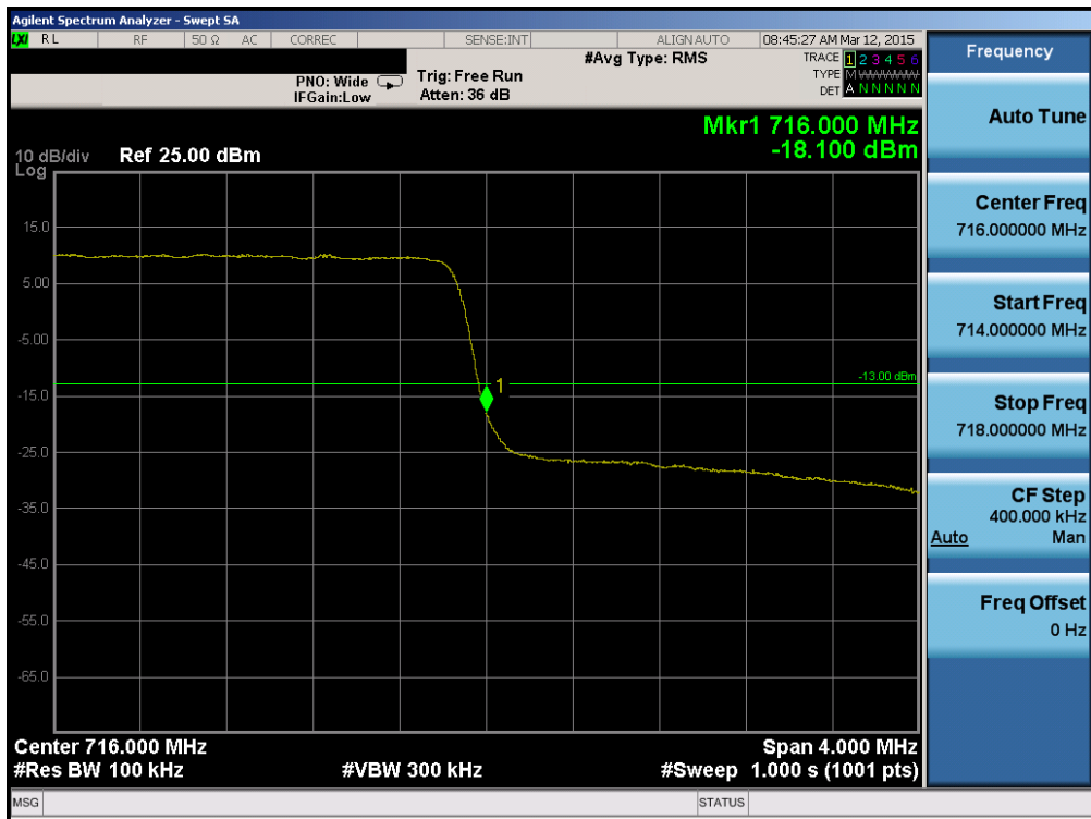
Plot 6-63. Upper Band Edge Plot (Band 12 - 3.0MHz QPSK - RB Size 15)
