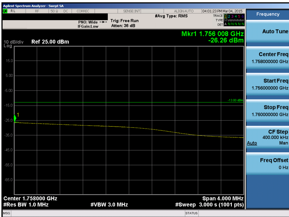
Plot 6-91. Upper Extended Band Edge Plot (Band 4 – 20.0MHz QPSK – RB Size 100)
