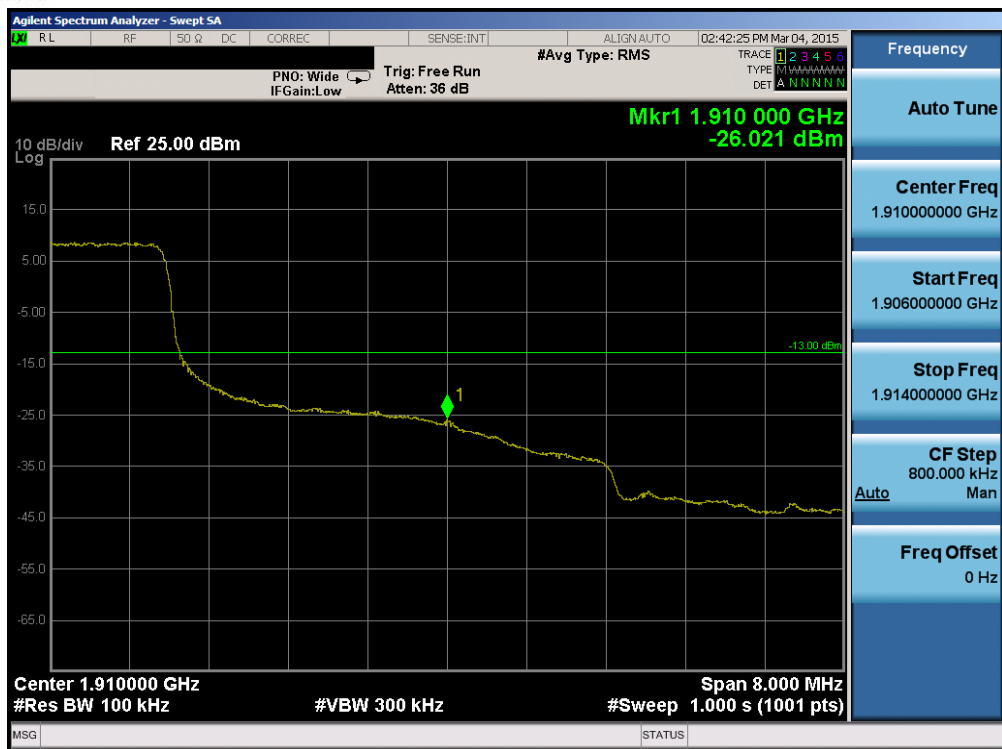
Plot 6-106. Upper Band Edge Plot (Band 2 – 10.0MHz QPSK – RB Size 50)
