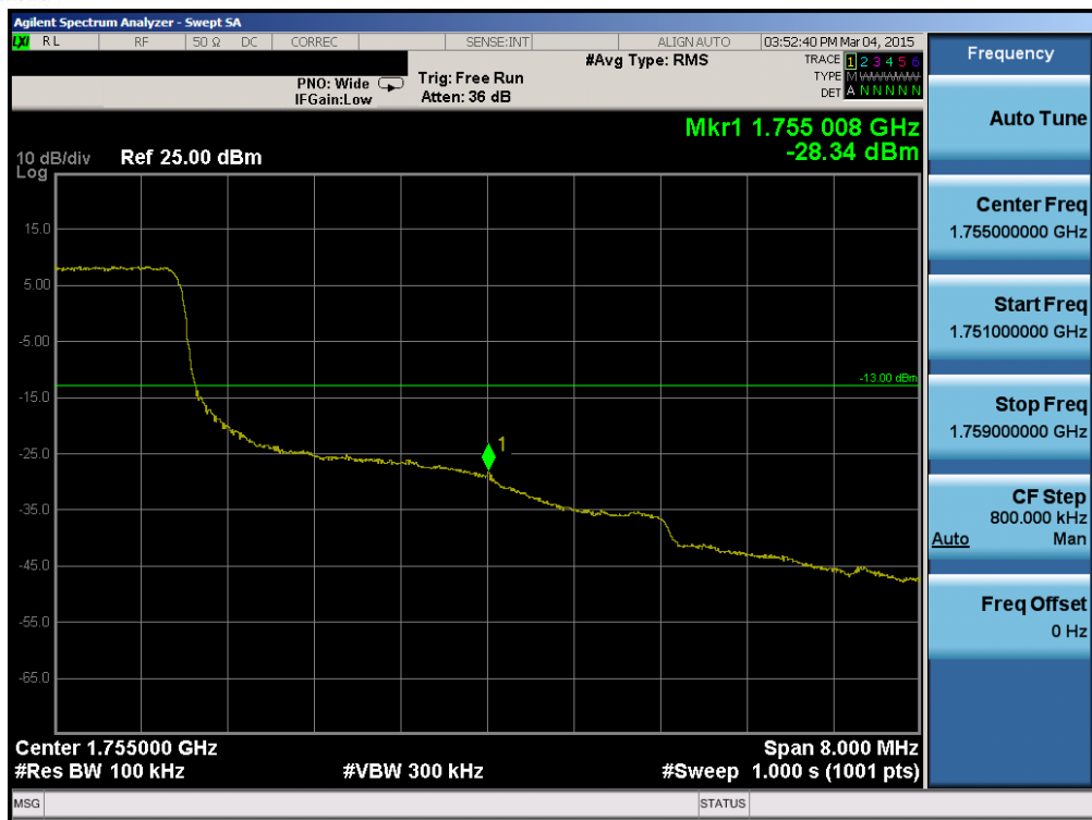
Plot 6-82. Upper Band Edge Plot (Band 4 – 10.0MHz QPSK – RB Size 50)
