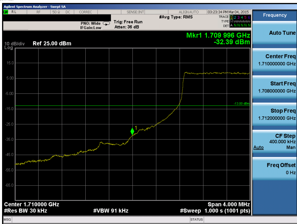
Plot 6-72. Lower Band Edge Plot (Band 4 – 3.0MHz QPSK – RB Size 15)
