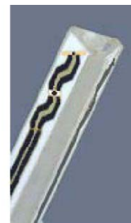
Figure 3.3 Probe Thick-Film Technique
