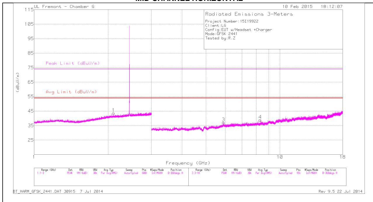
Note: Emission was scanned up to 26GHz; No emissions were detected above the noise floor which was at least 20dB below the specification limit.
