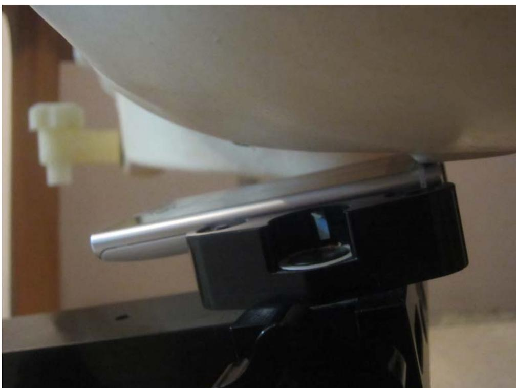
■ Test Setup Photo(Body SAR Test Photo)
