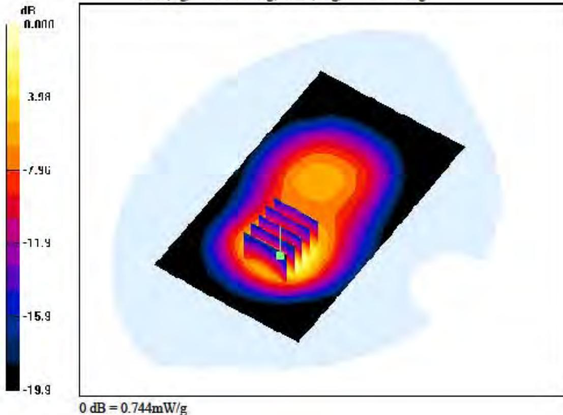
**DIGITAL EMC CO., LTD****DUT: LG-E400f; Type: Bar**
