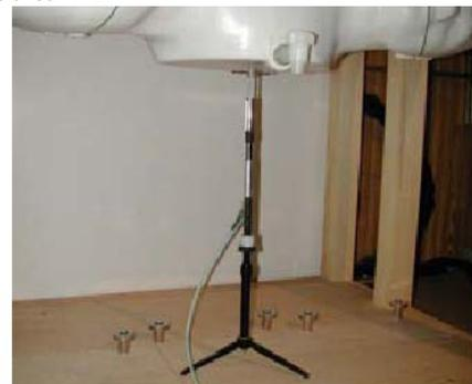
Figure 9.1 Dipole Validation Test Setup
