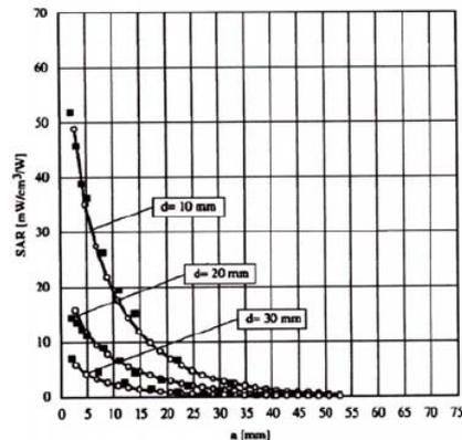
Figure 3.5 E-Field and Temperature Measurements at 1800MHz
