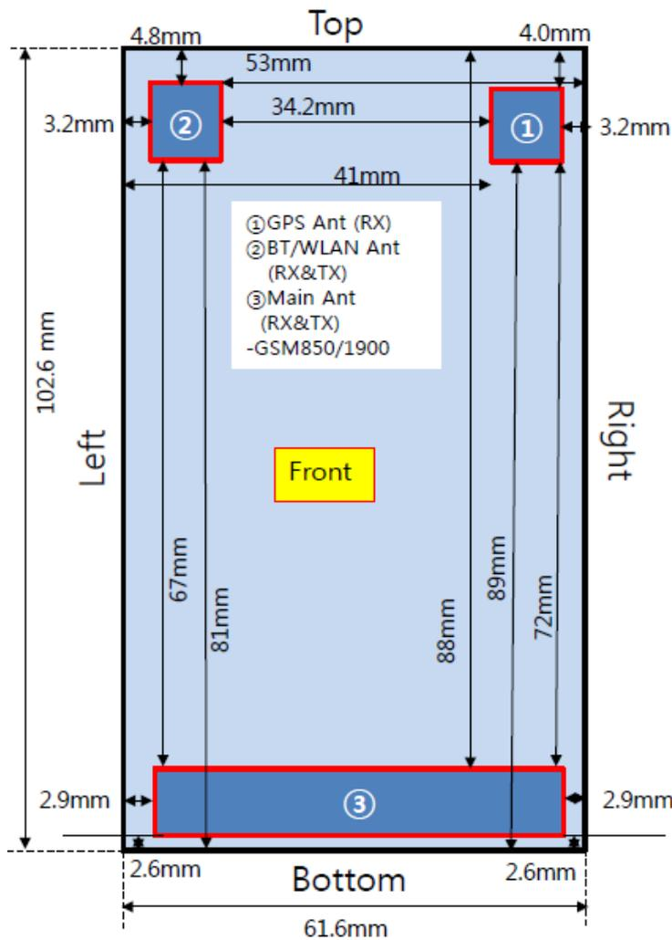
Figure 13.1 Identification of Sides for SAR Testing
