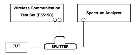
(Configuration of conducted Emission measurement)
