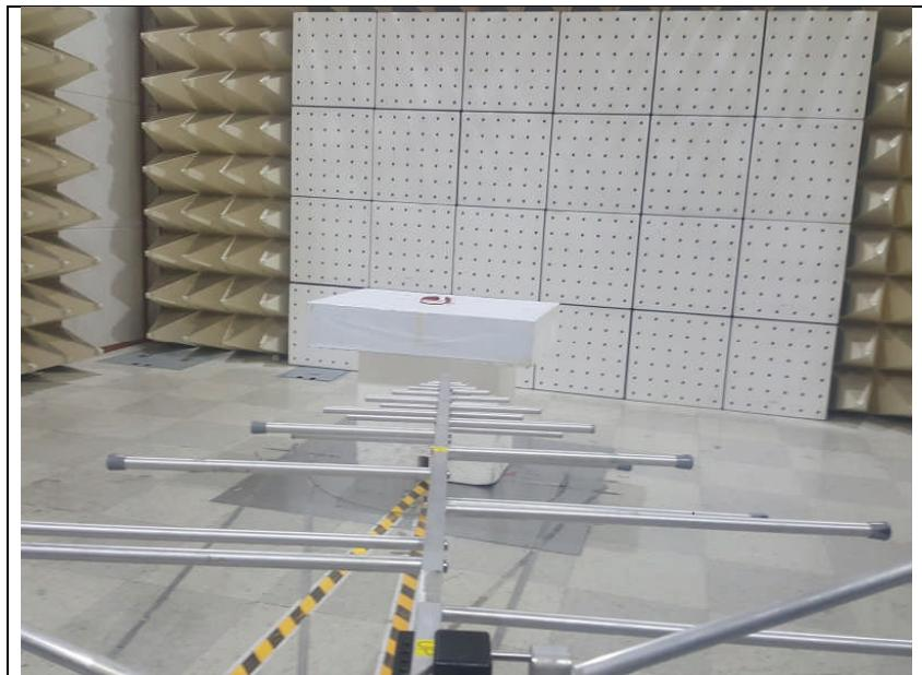
**3. Photo of Radiated Spurious Emission Test (Above 1 GHz)**
