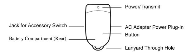
An optional accessory switch can be used with RCx-Txm and it's work is same as the button on RCx-Txm.
