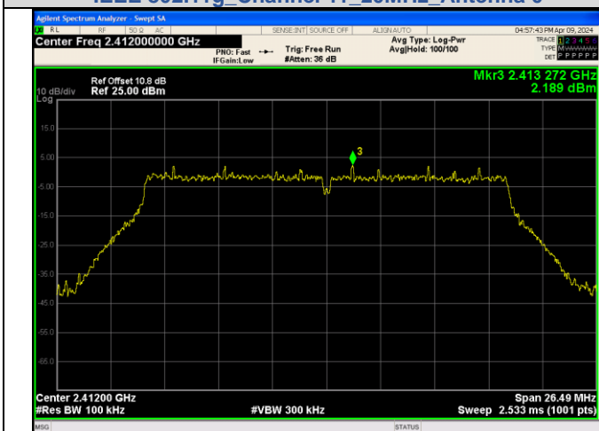
In-Band Reference Level IEEE 802.11n Channel 1 20MHz Antenna 0
