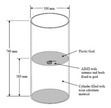
For the testing, the equipment under test (EUT) was suspended in a Plexiglas torso simulator as specified above. The simulator used was constructed in accordance with FCC 95.639(a)(2)(i), EN 301 839-1 (A.113) and EN 301 489-27 annex B.
