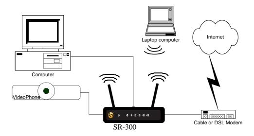
Figure 1 - Basic Network Configuration
