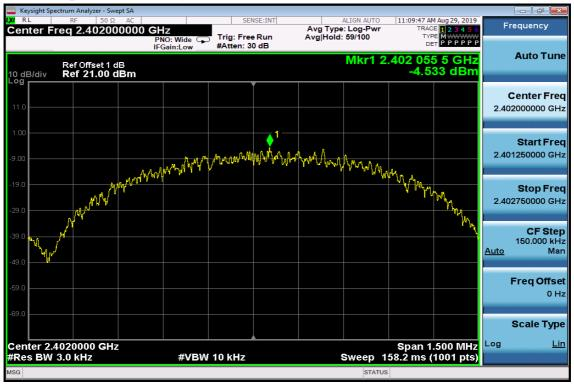
**Power Spectral Density Test Plot (CH-Mid)**
