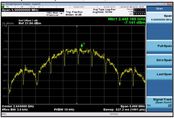
**Power Spectral Density Test Plot (CH-High)**
