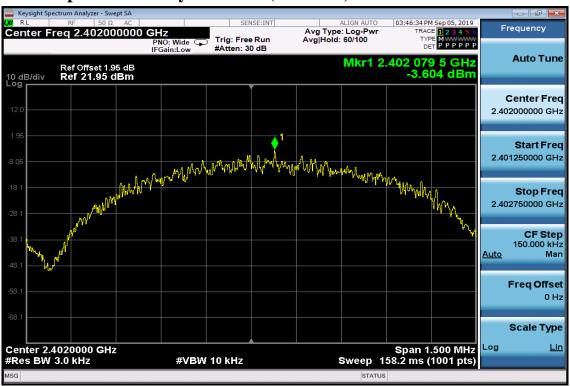
Power Spectral Density Test Plot (CH-Mid)
