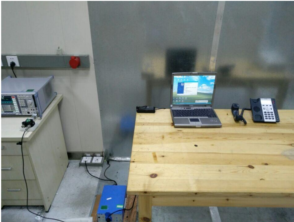
FCC RADIATED EMISSION TEST SETUP BELOW 1GHZ
