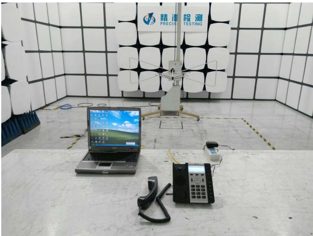
FCC RADIATED EMISSION TEST SETUP BELOW 1GHZ
