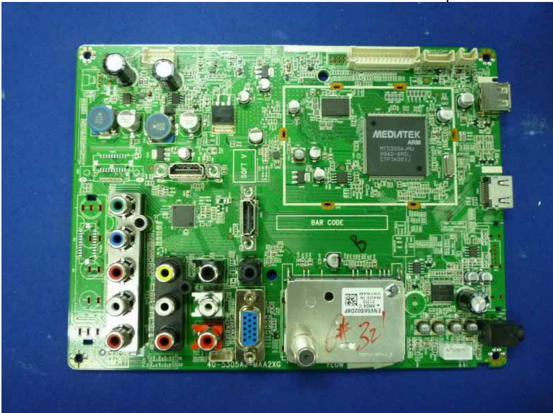
Figure 16 Component Side of the PCB
