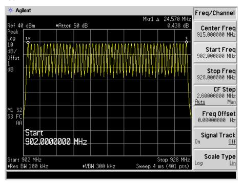
For GFSK mode Channel Spacing Low Channel CH=500 kHz
