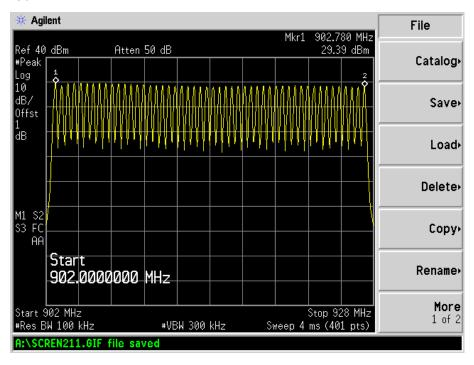
For GFSK mode Channel Spacing Low Channel CH=500 kHz
