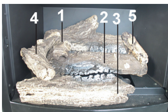
FIG (16) STEP 5: Insert the recessed hole on the bottom of log 5 onto the pin on log 1, with the other end of log 5 placed on log 2, as shown.
