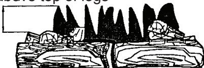
Figure 37 - Correct Flame Pattern with heater set to High Flame
