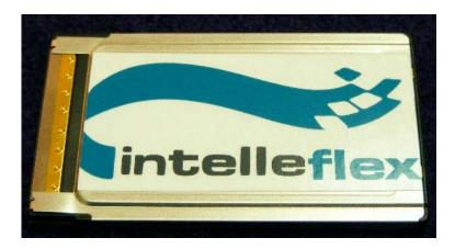
The MMR6500 reader is designed in a PCMCIA/PC card mechanical format for integration into handheld and mobile RFID readers. The reader uses standard PC card connectors, but the electrical interface is a non-standard, proprietary serial interface that cannot be used in standard PC card slots in laptops or general computing devices.
