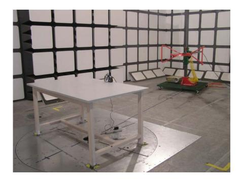
Charging Mode: Radiated Emission – Rear View (30-1000MHz)
