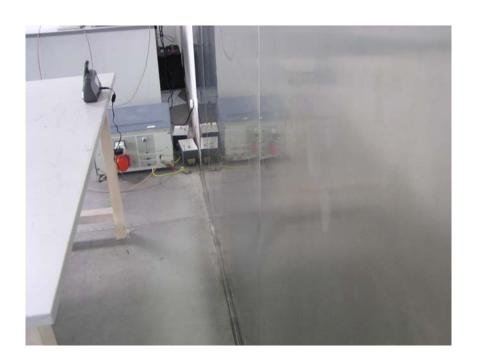
Charging Mode: Radiated Emission – Front View (30-1000MHz)
