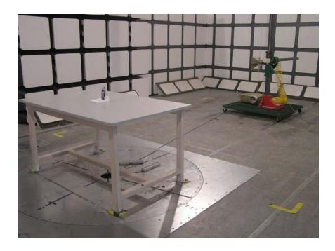
Radiated Emission - Rear View (Above 1000MHz)
