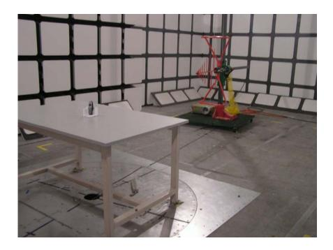
Radiated Emission – Rear View (30-1000MHz)
