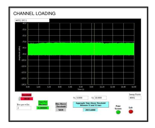
The level of traffic loading on the channel by the EUT is 20.156%
