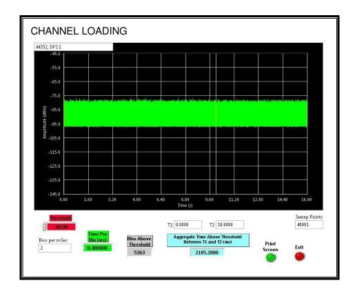
The level of traffic loading on the channel by the EUT is 21.052%
