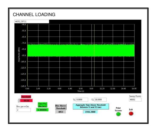
The level of traffic loading on the channel by the EUT is 19.412%
