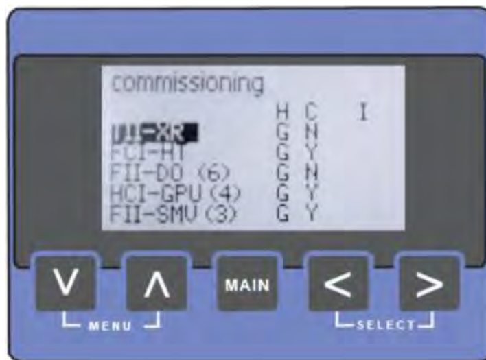
FIGURE 4-13 The board list screen (commissioning)
