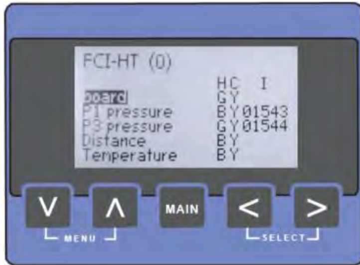
FIGURE 4-14 The function list screen (commissioning)
