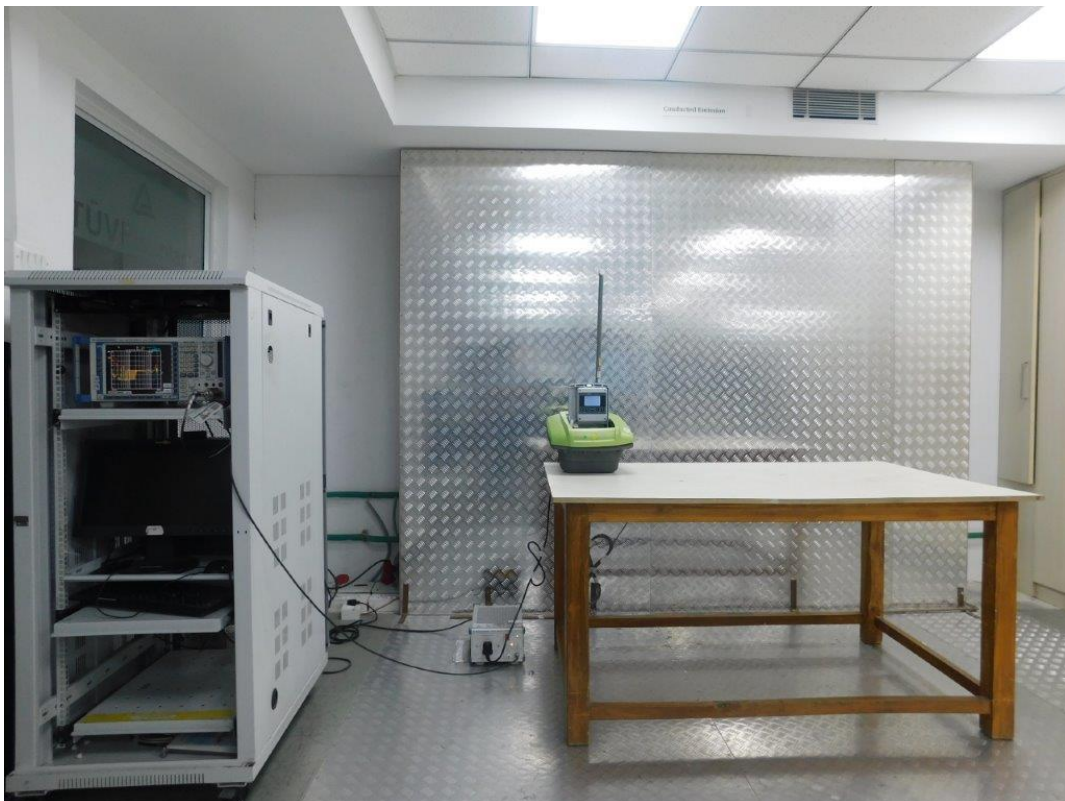
Conducted emission test on AC power line test setup photo
