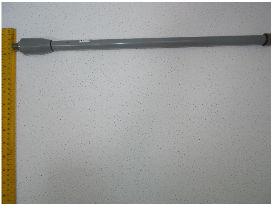
Antenna 4: HGV – 2409 U Omni antenna ( 8 dBi)
