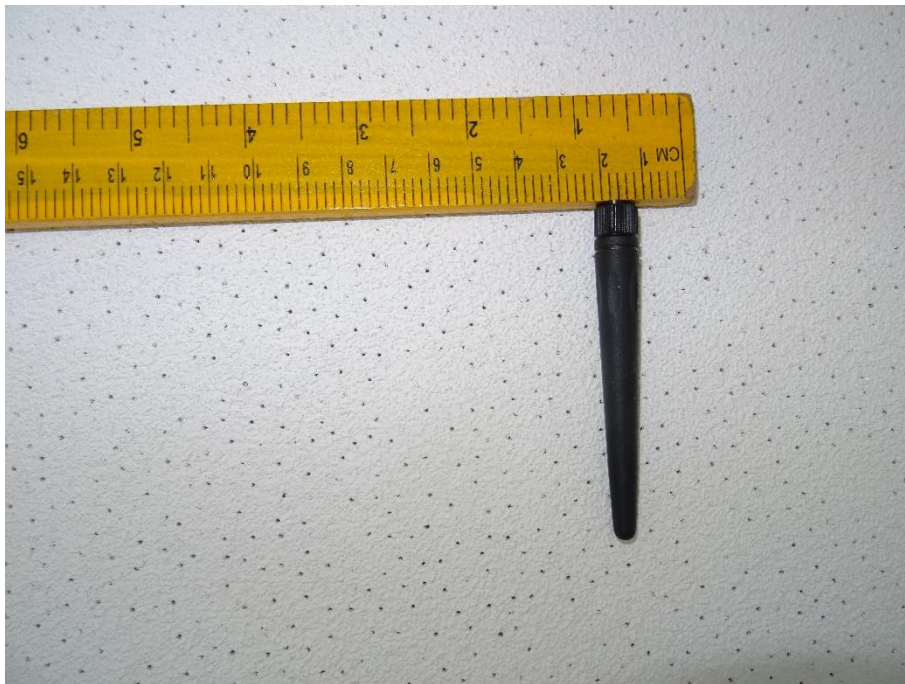
Antenna 1: HG2402RDR-RSP / Rubber Duck Omni antenna (2 dBi)
