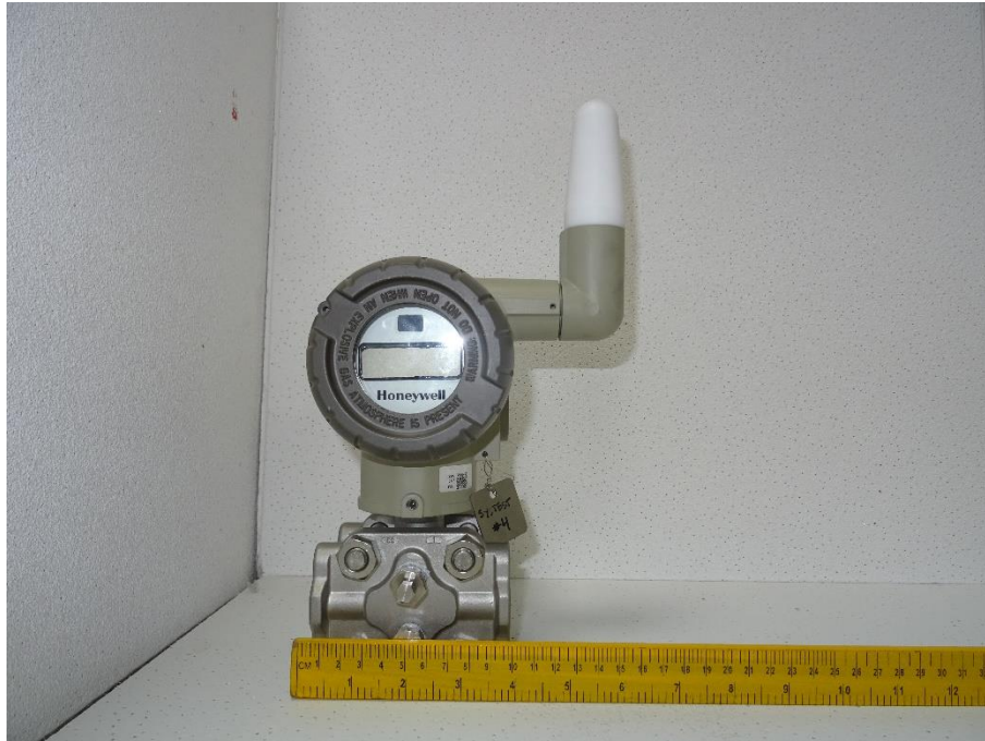
Photo 7: Dimensional view of Host with - 2 dBi antenna
