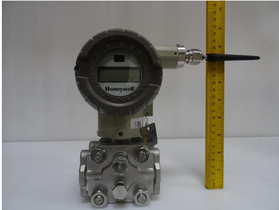
Photo 11: Host with +2 dBi antenna (front view)
