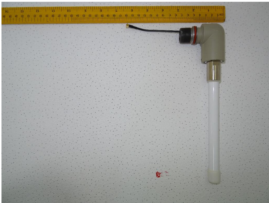
Antenna 2: EM-B14503-MMP-Z6 antenna (4 dBi)
