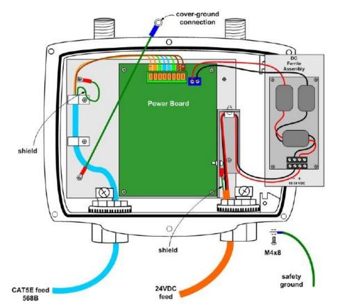
Figure 7: Ethernet and field DC power
