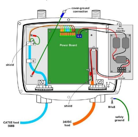
Figure 7: Ethernet and field DC power
