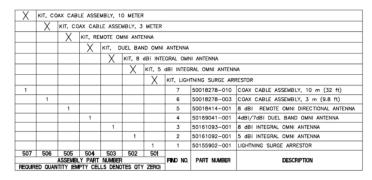
Figure 3: Antenna components
