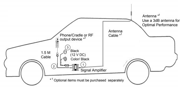
Typical Installation For Under The Seat Mounting
