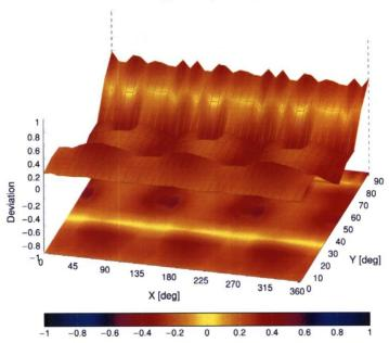
Probe isotropy for E<sub>tot</sub>: probe rotated  $\phi=0^\circ$  to 360°, tilted from field propagation direction  $\vec{k}$  Parallel to the field propagation ( $\psi=0^\circ-90^\circ$ ) at 30 GHz: deviation within  $\pm 0.39$  dB Parallel to the field propagation ( $\psi=0^\circ-90^\circ$ ) at 60 GHz: deviation within  $\pm 0.46$  dB
