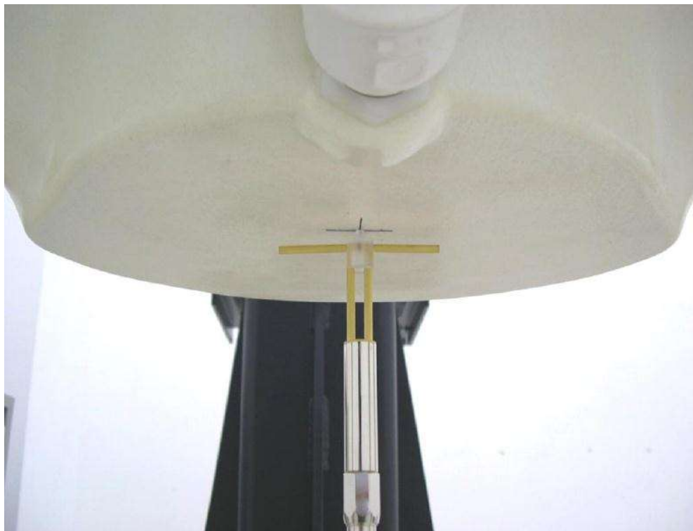
Picture 8.2 Photo of Dipole Setup
